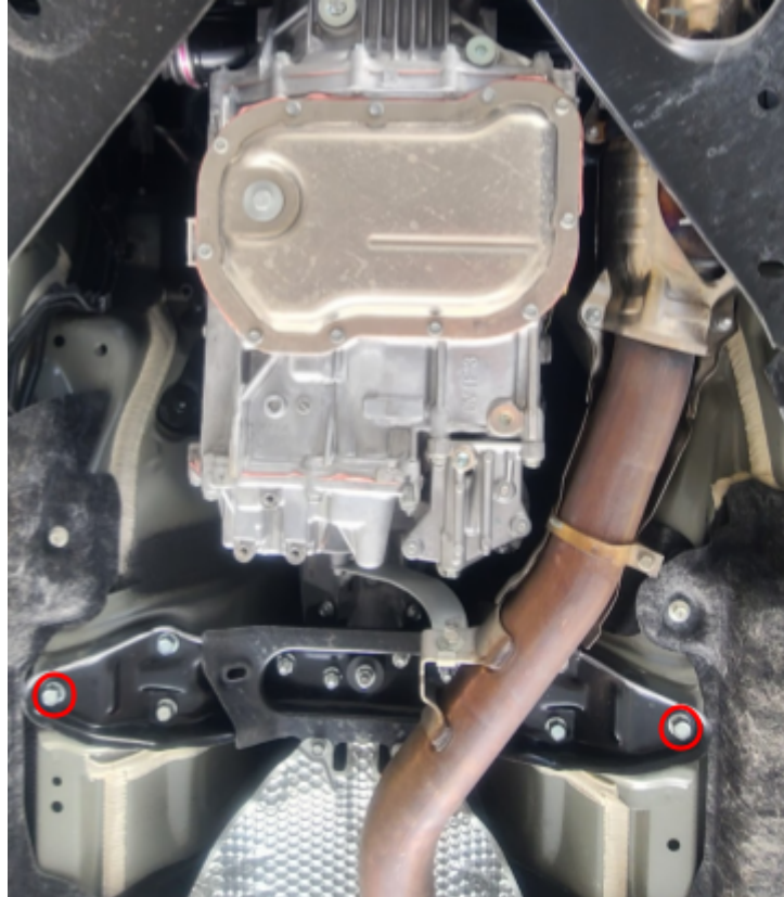
Figure 1: Bottom View Bolts to Remove.
