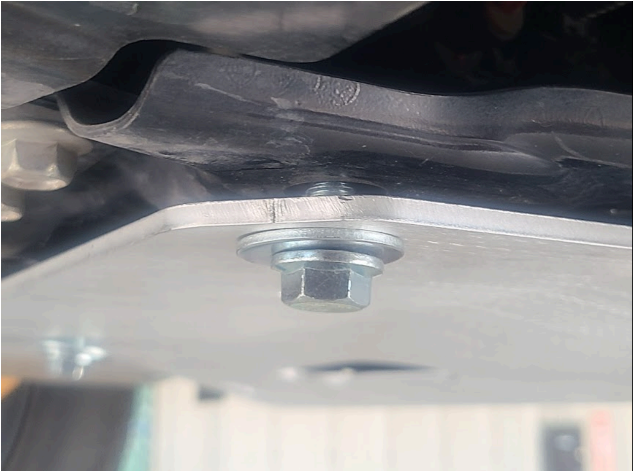
Figure 6: Engine Skid Spacing Compatibility.
