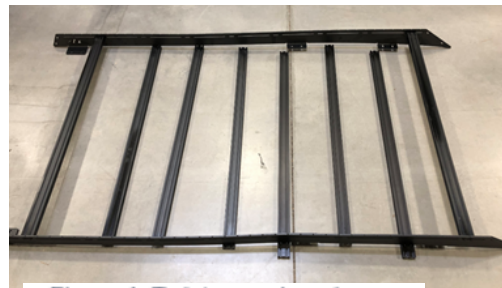
Figure 4: T-slot cross bars lay out
