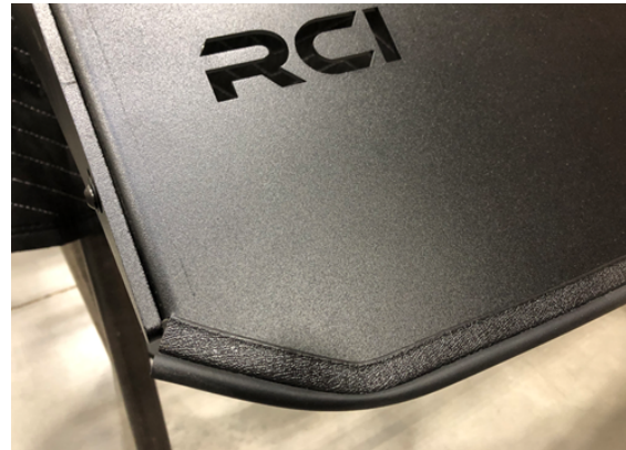
Figure 10: Front fairing weather strip install
