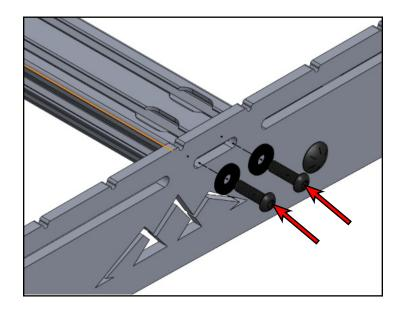
**Note:** RCI's roof racks are designed to have the aluminum T–Slot cross bars mounted to the small oval cutouts on the side panels (as shown). However, there may be a need for them to be shifted to other positions to accommodate third-party accessories.
