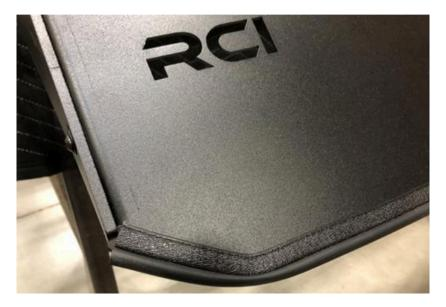
37. Use the included 1/4" washers, button head bolts, and keps nuts to loosely secure the front fairing to the rack assembly.
