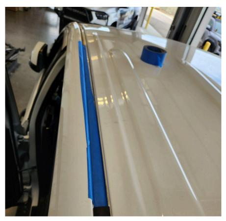
9. From the rear of the roof, measure 8-1/8" and mark
