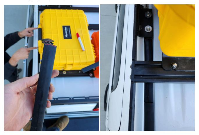
d. Lay the remaining strip within the channel at the front of the vehicle, aligning the tab on the underside of the stripping with the locating "clamps" within the channel. Repeat the process of marking and trimming the stripping to fit.
