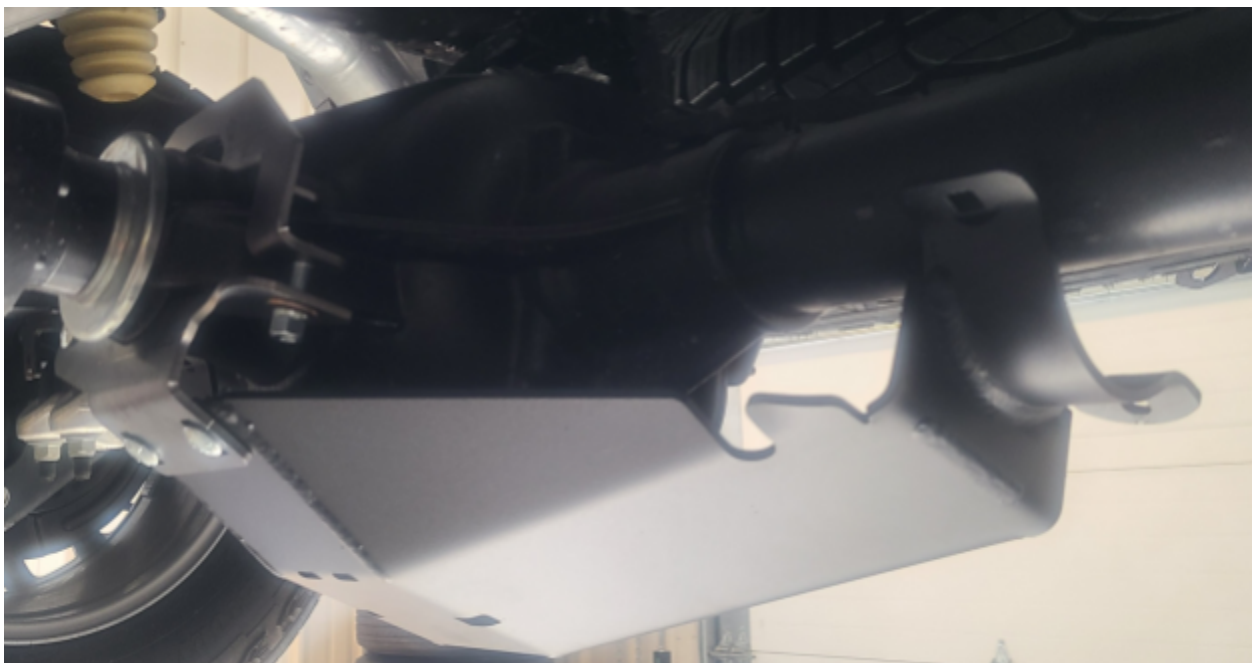
Figure 3: Assembled Diff Skid Install
