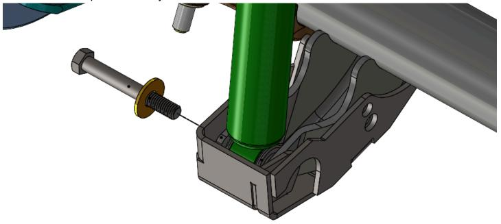
4. Loosely install a washer and nut on the threaded end of the bolt from the previous step.
