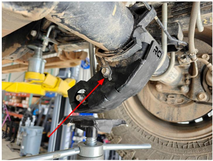
6. Repeat the process of installing the driver side shock mount using the included 1/2x3.75 bolt, washers, and nut.
