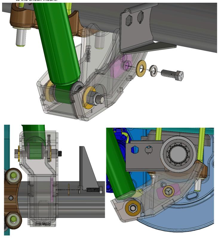
8. Tighten all hardware and torque the shock mounting hardware to factory specifications.
