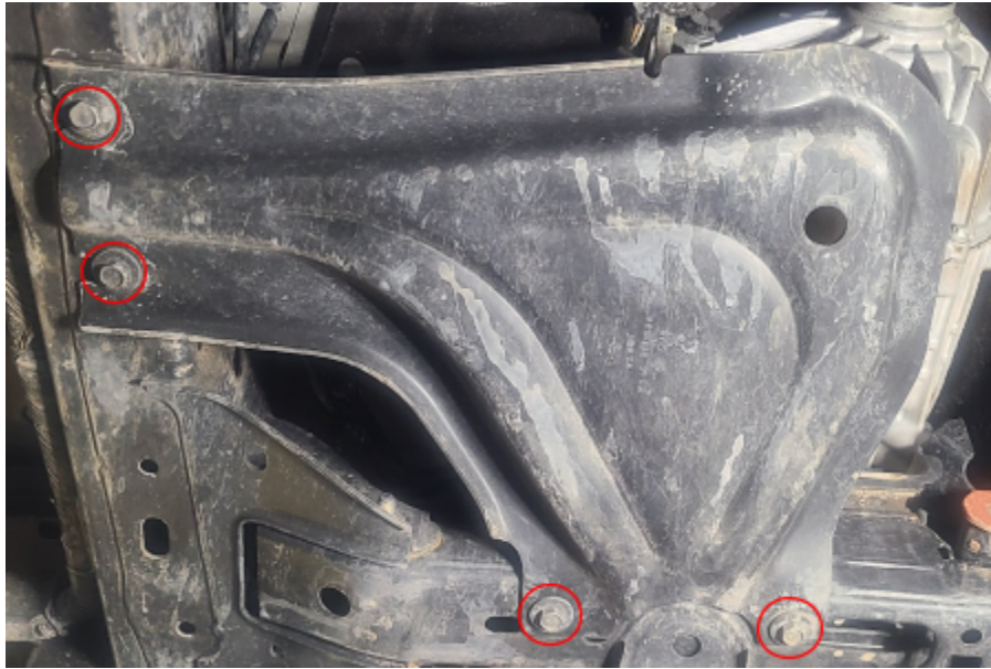
Figure 1: OEM Hardware Removal
