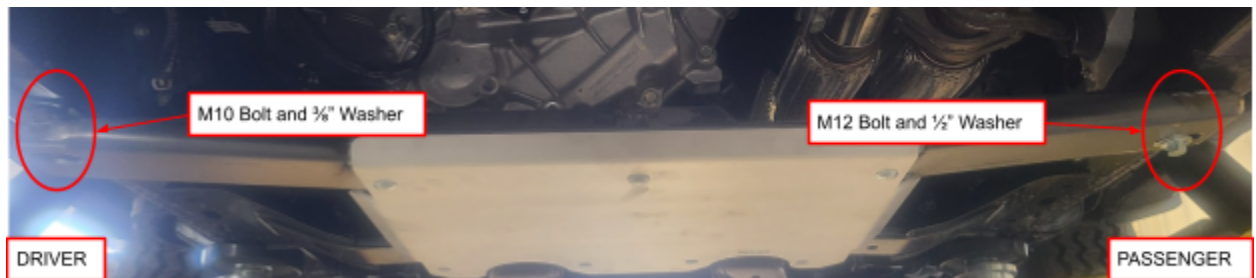
Figure 6: Cross Member Hardware Install
