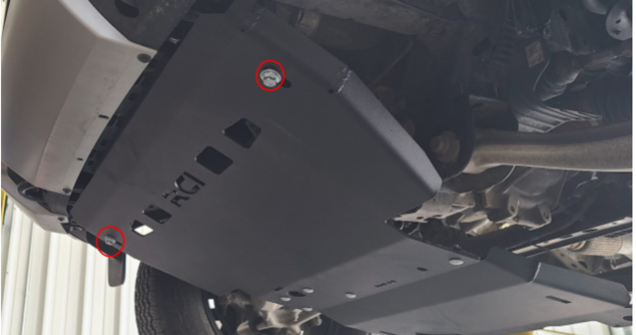
Figure 4: Front Hardware Install
