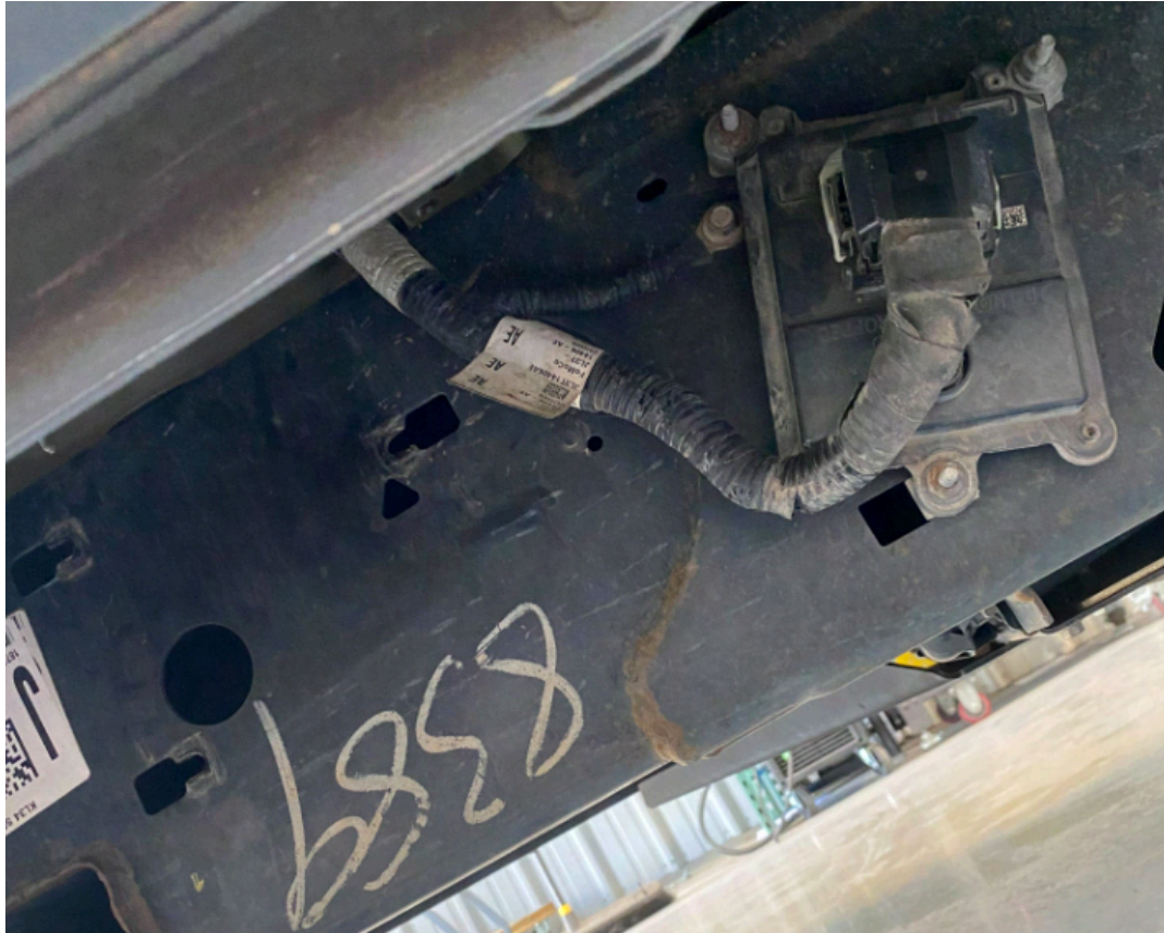
Correct Relocation of Fuel Control Box
