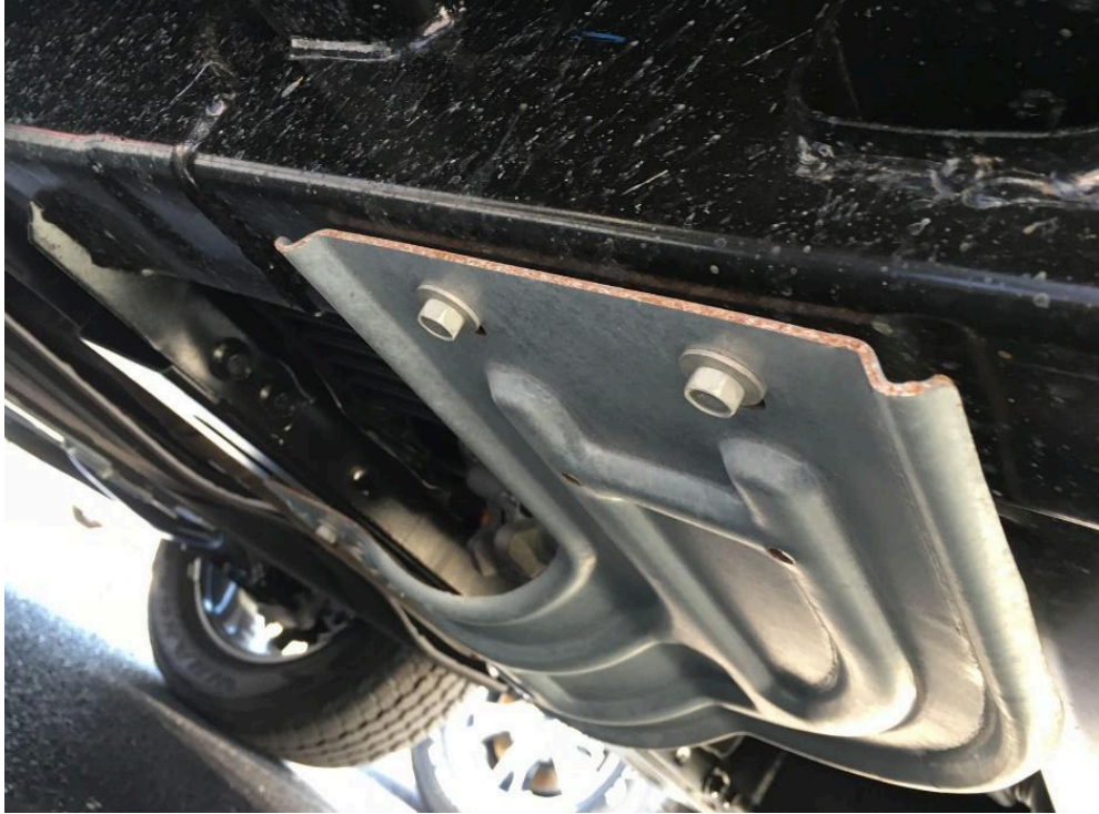
OEM Transfer Case Skid to be Removed.
