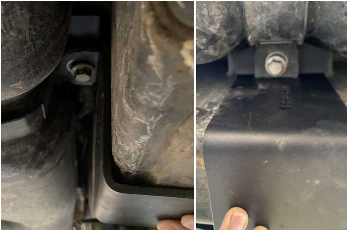
Reinstallation of Fuel Strap
