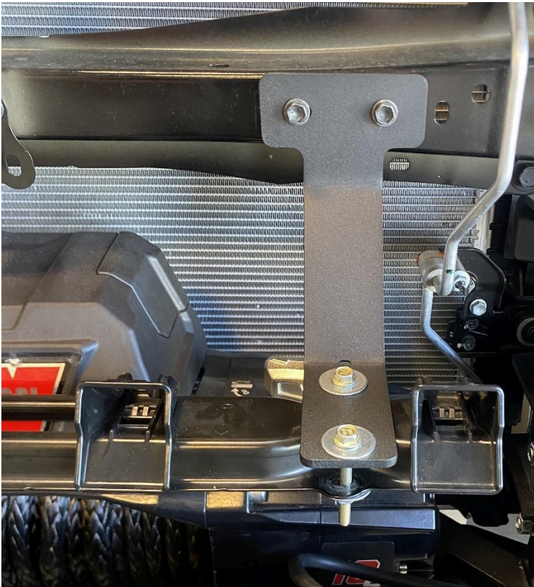
Figure 26: Correctly installed support bracket.
