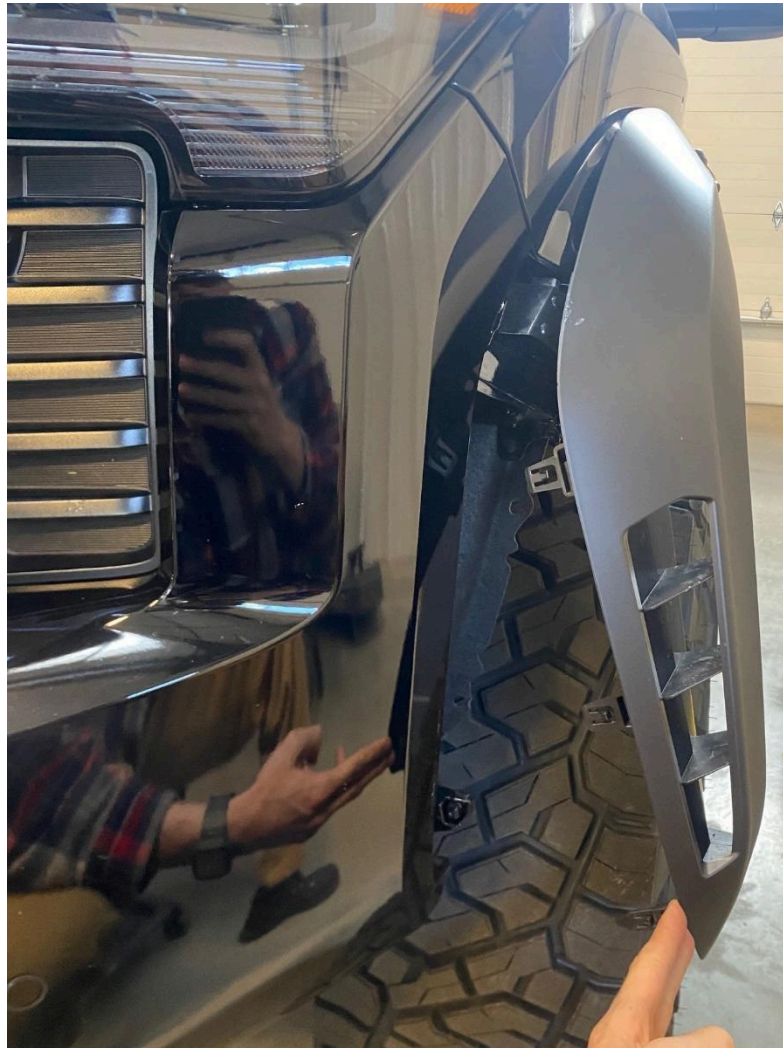
Figure 7: Pull back fenders.
