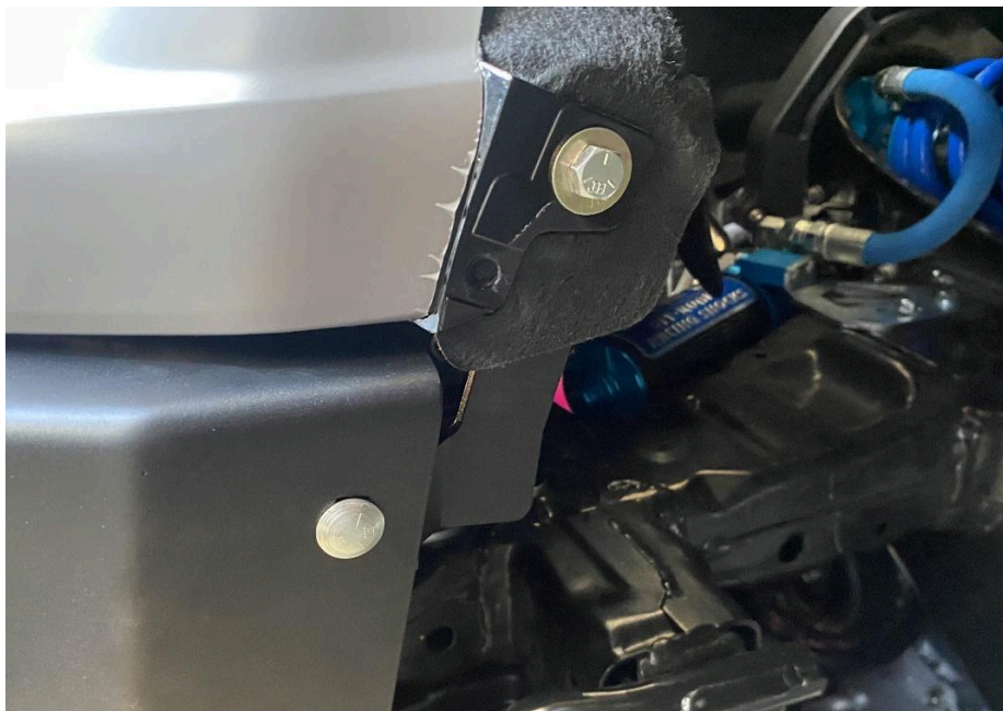
Figure 28: Correct installation of Driver side trim bracket.
