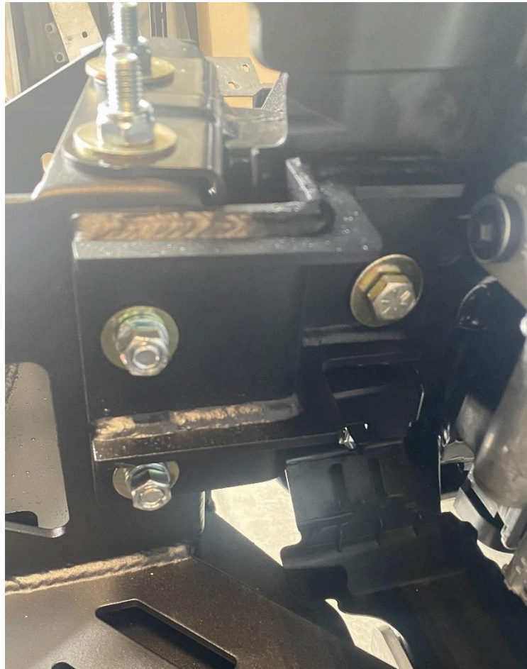
Figure 23: Correct installation of secondary bracket.
