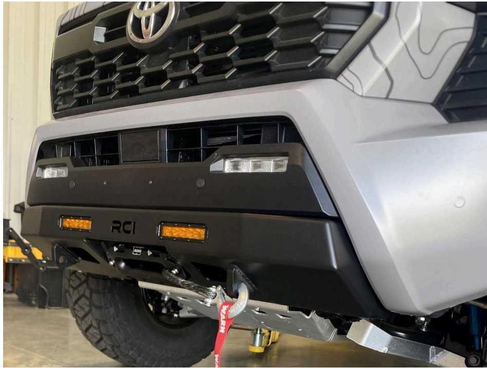
Figure 27: Correct bumper installation.
