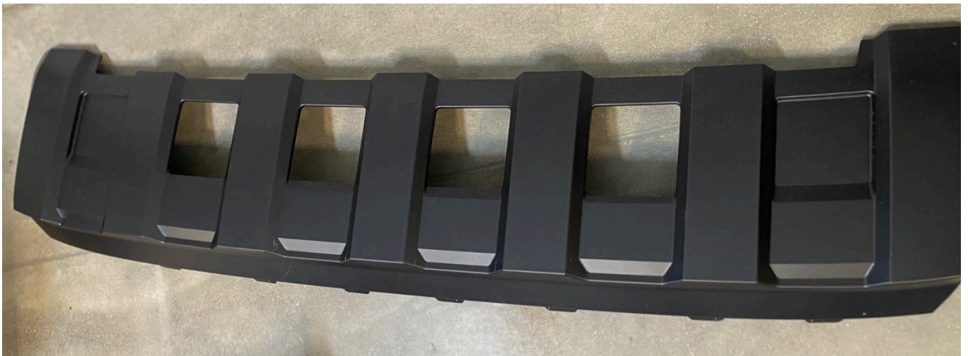
Figure 15: Lower bumper cover.
