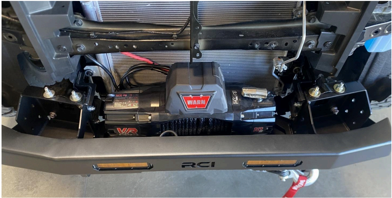
Figure 24: Example of winch and lights installed.
