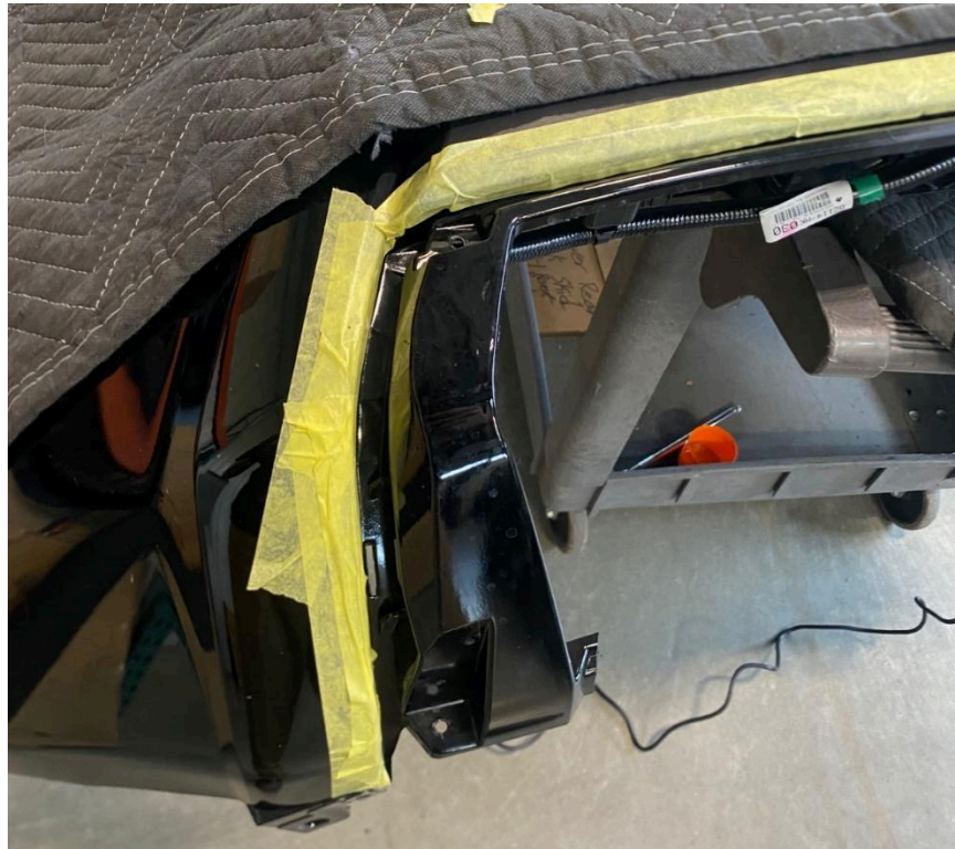
Figure 16: Tape off bumper.
