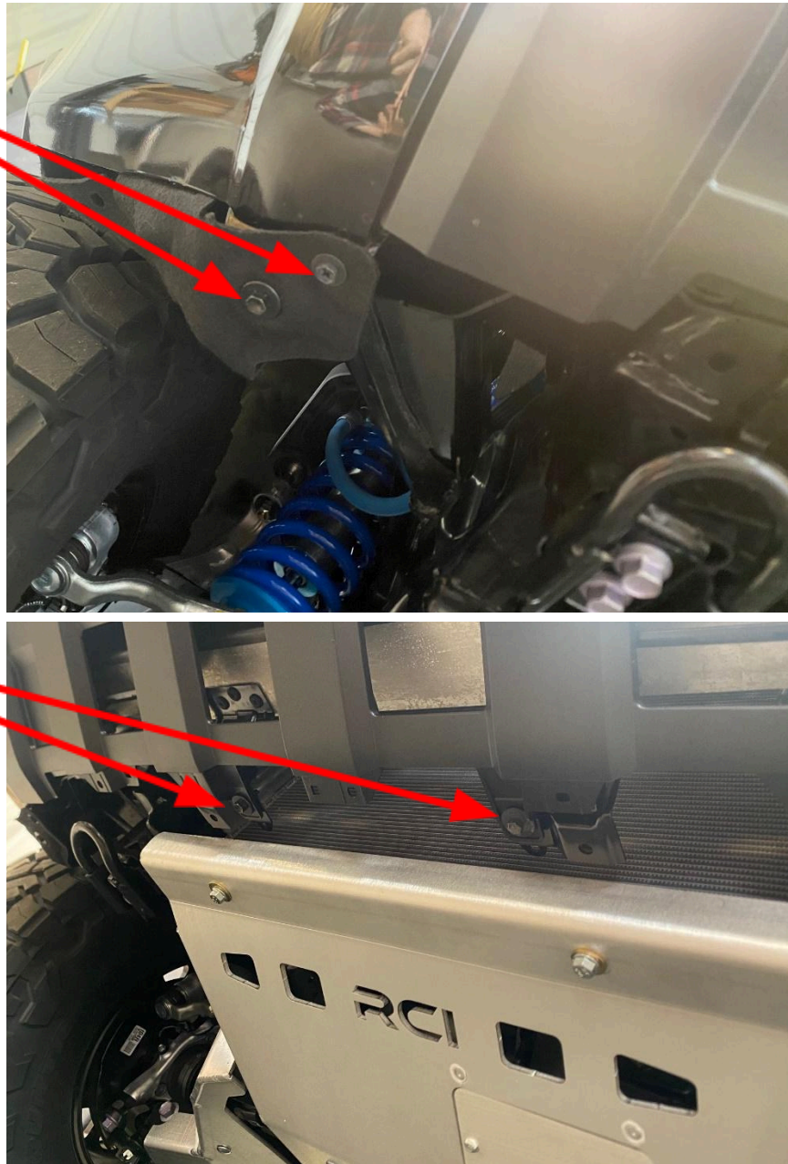
Figure 5: Remove underside fasteners.
