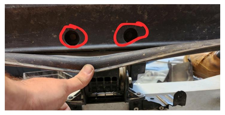
c. Remove the 2 bolts securing the air dam motor module to the bottom of the aluminum crash bar.
