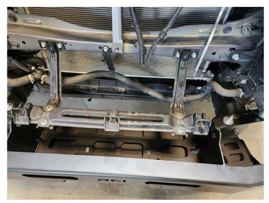
44. Lift the OEM bumper with the plastic tabs on the OEM bumper with the slots in the black bracket installed in the previous step. Push the OEM bumper backwards and into the vehicle.
