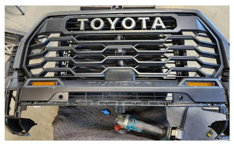
24. Follow the cut line up to match the inner flat of the slot
