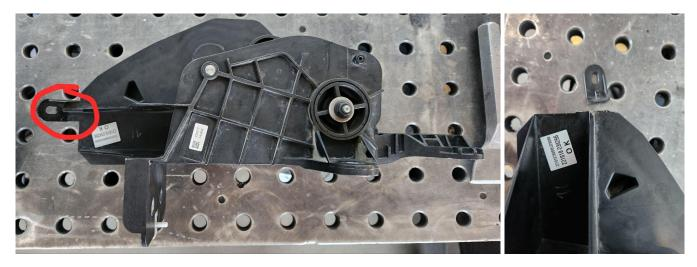
j. Remove the large flange originally used to attach the module to the aluminum crash bar
