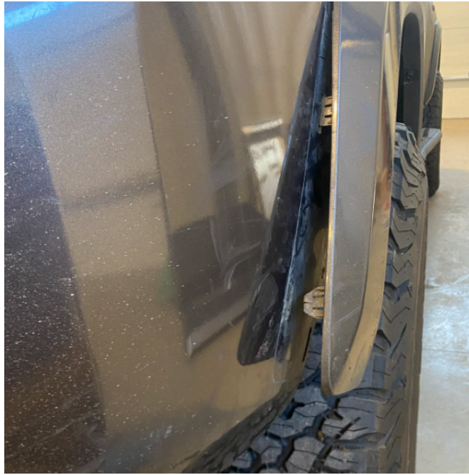
Figure 8: Lower fender pulled away.
