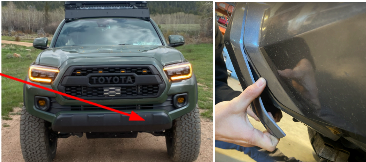
Figure 2: OEM bumper cover
