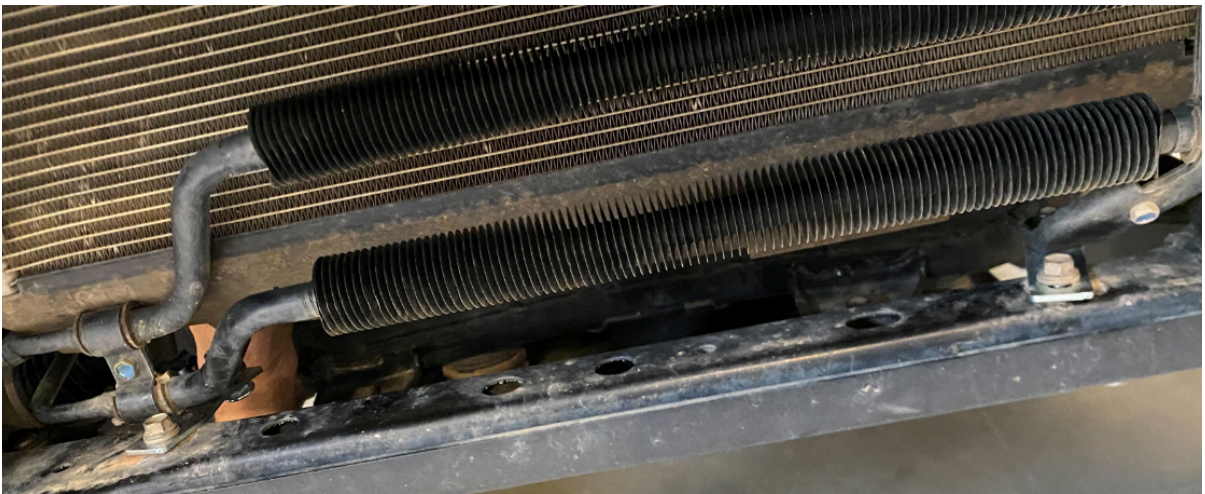
Figure 17: Correct installation of frontmost brackets.
