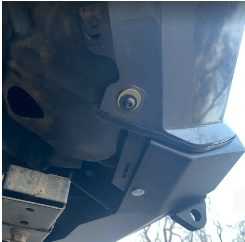
Figure 27: Correct installation of trim bracket
