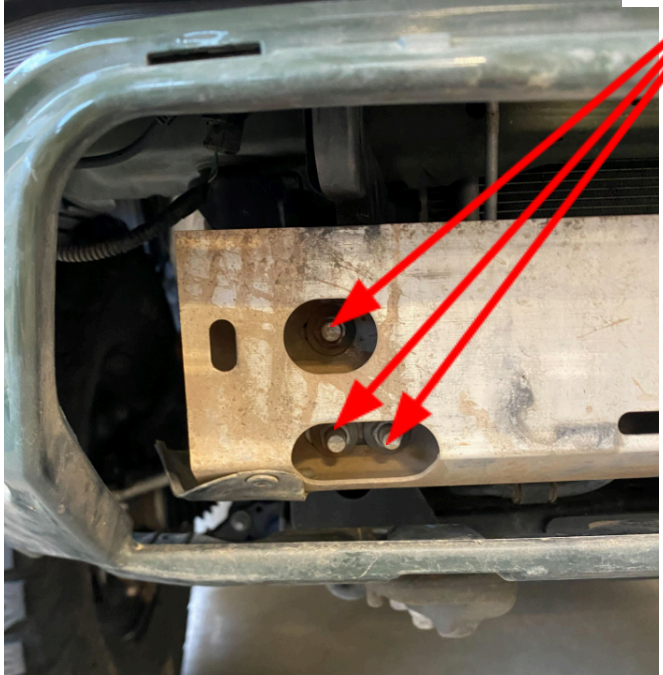
Figure 4: OEM Crash bar to be removed.
