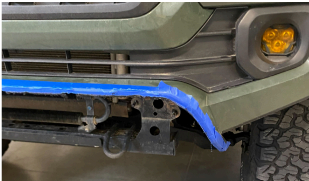
Figure 13: Bumper after cut
