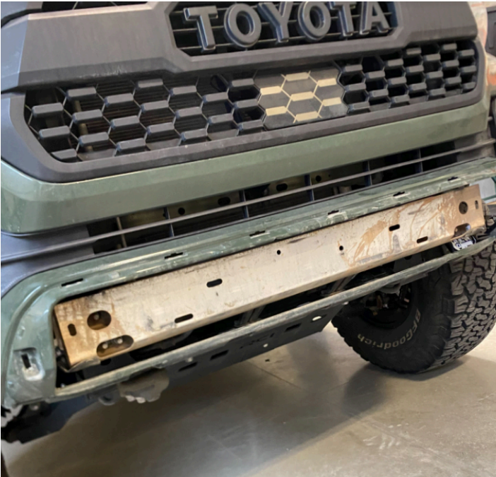
Figure 4: OEM Crash bar to be removed.
