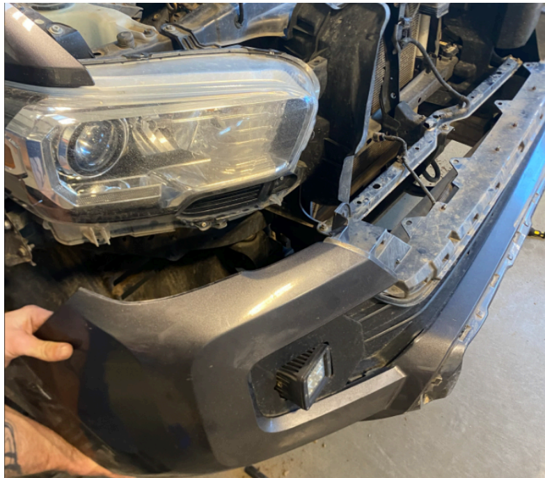
Figure 9: Example of the bumper half removed.
