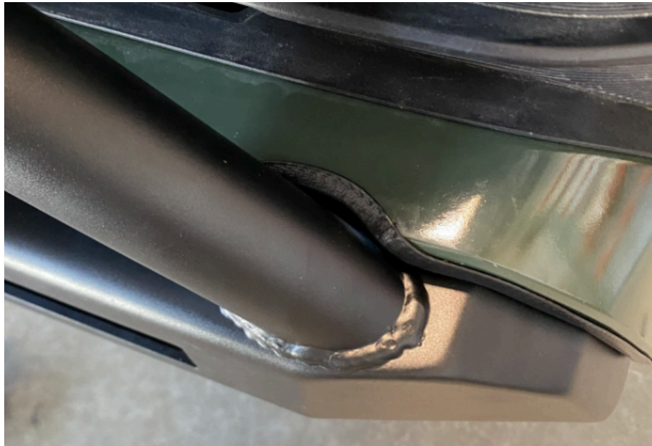
Figure 21: Example of finished cut for hoop.
