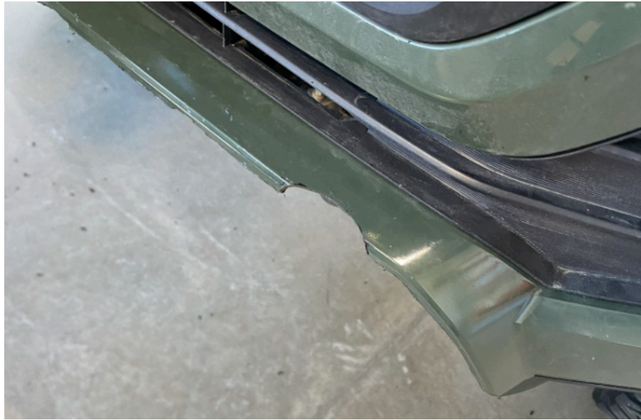
Figure 20: Example hoop clearance cut.
