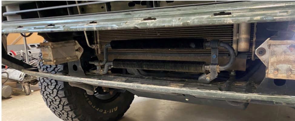
Figure 10: Remove crash bar brackets.
