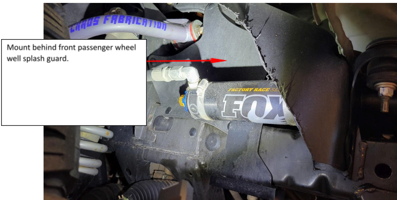
Figure 9: Mount located behind passenger wheel well splash guard.
