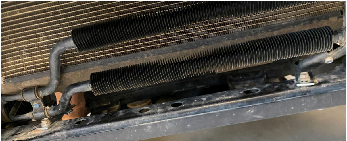
Figure 14: Correct installation of frontmost brackets.
