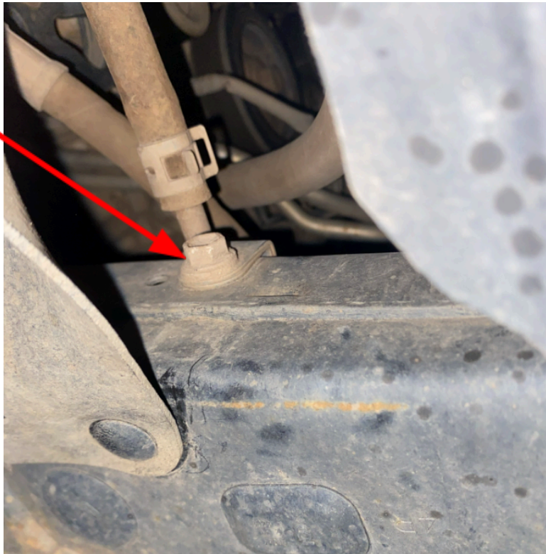
Figure 10: Mount located behind passenger wheel well splash guard.
