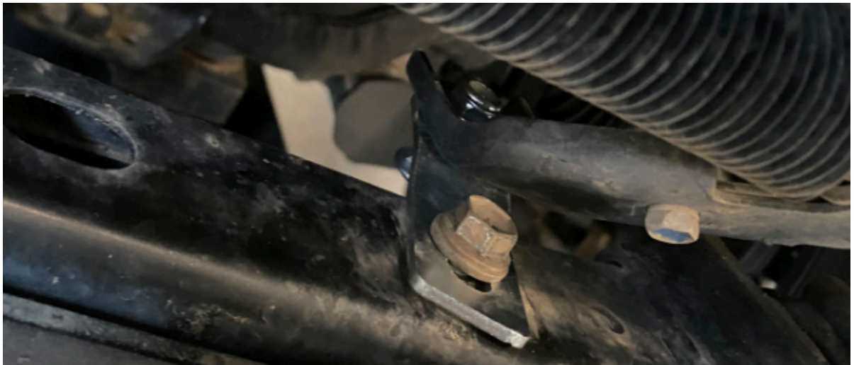
Figure 13: Correct installation of frontmost brackets.
