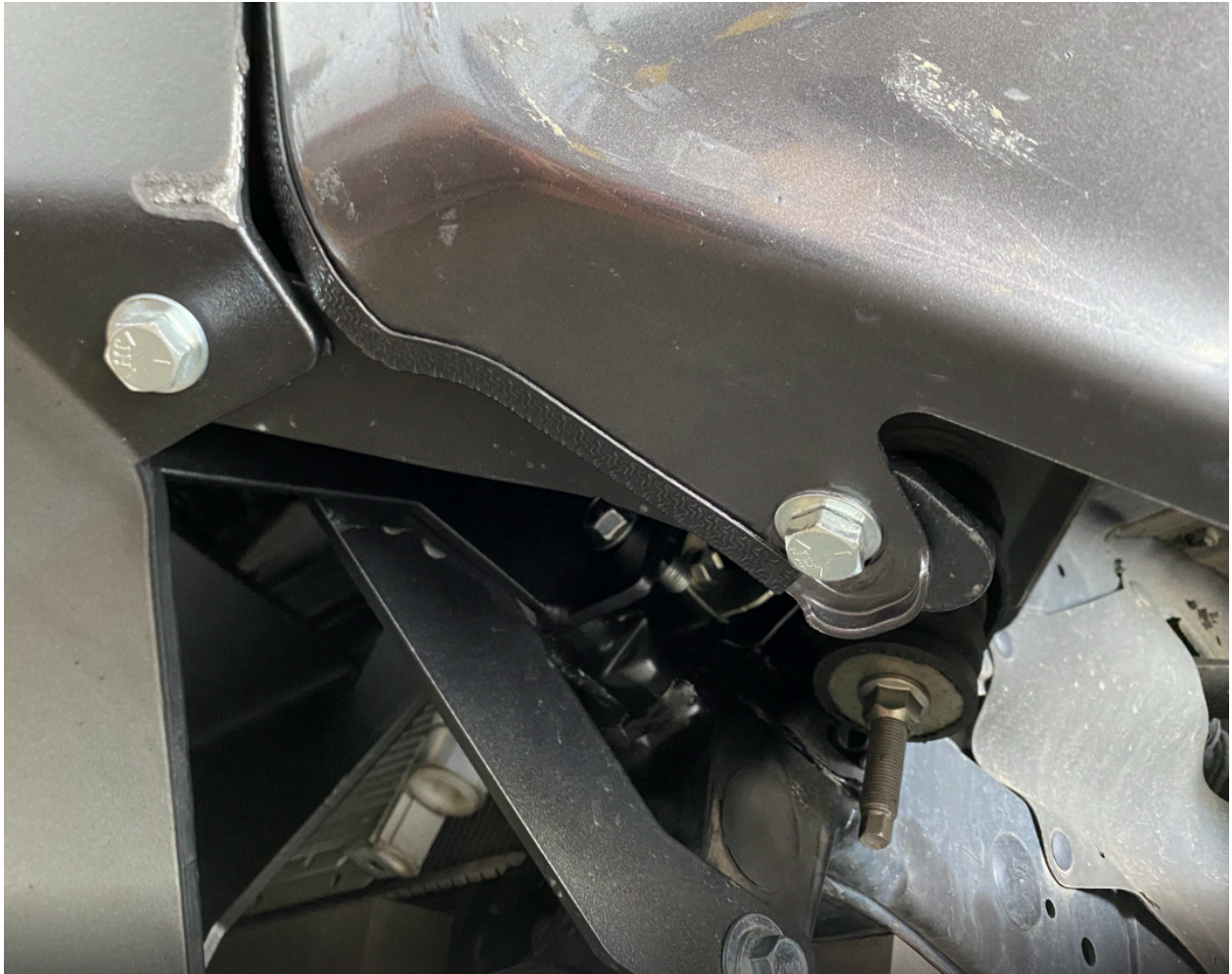
Figure 20: Correct installation of Support Bracket
