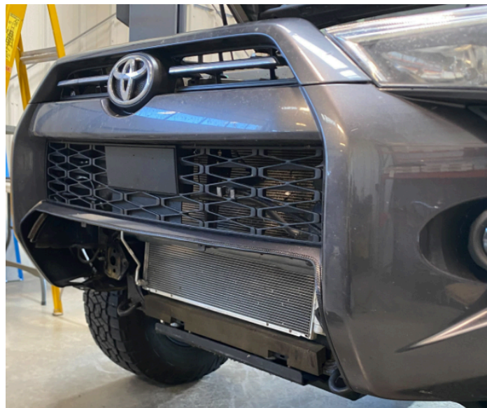
Figure 13: Vehicle with cut bumper reinstalled
