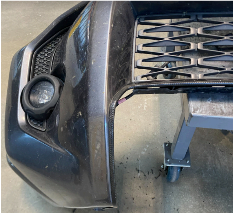
Figure 12:Finished cut with trim installed.
