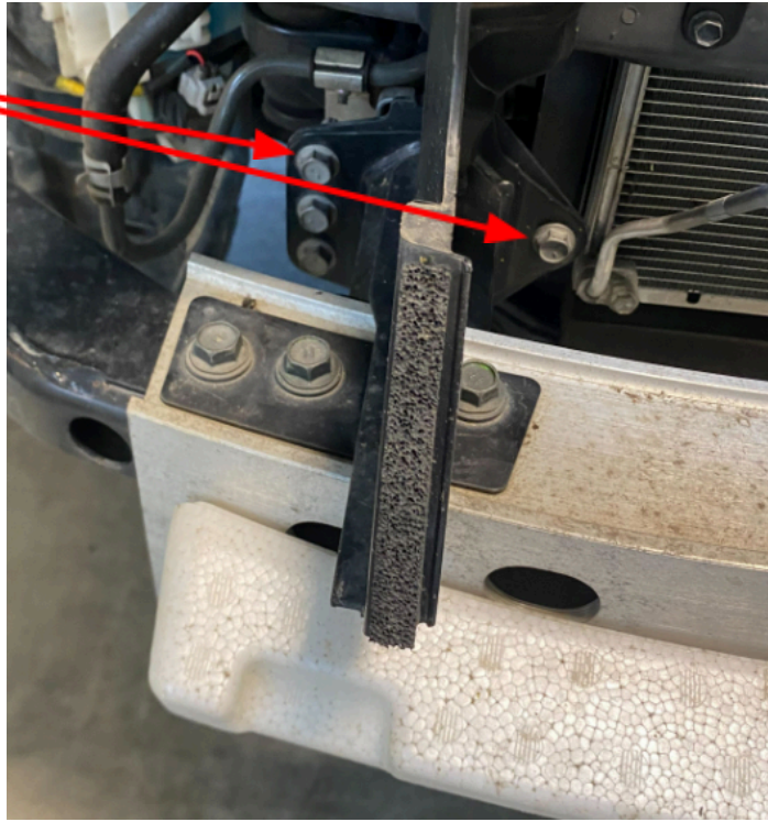
Figure 6: OEM crash guard to remove.
