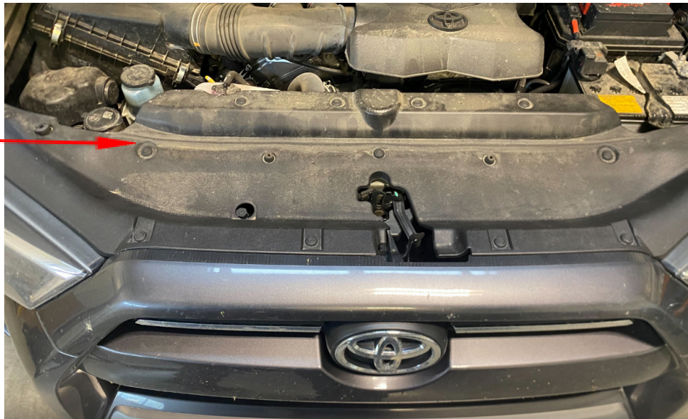
Figure 1: Clips and trim to be removed.
