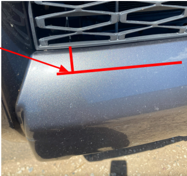
Figure 9: Cut line location.
