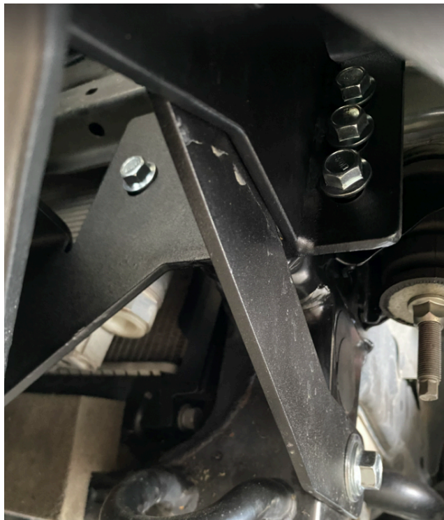
Figure 16: Correct installation of 14mm bolts.
