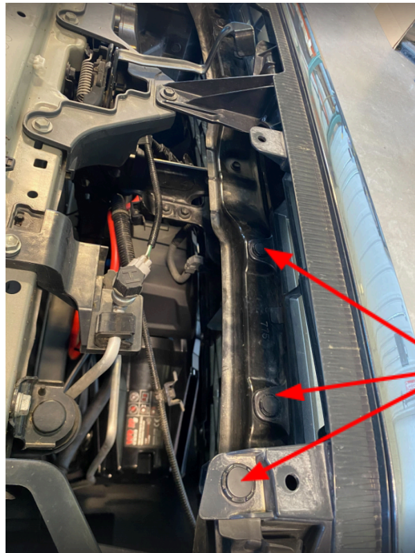
Figure 3: Clips securing grill to crossmember.
