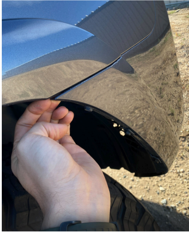
Figure 5: Start bumper removal from bumper corners.
