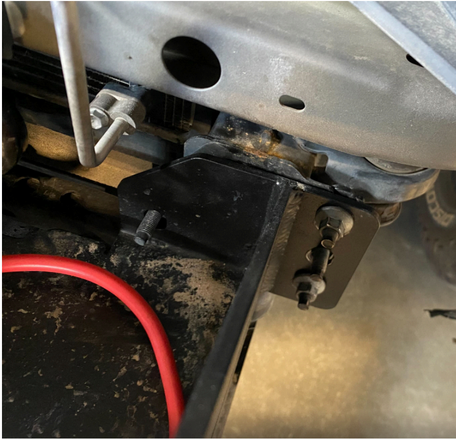
Figure 9: Correct installation of bumper on mounting surface
