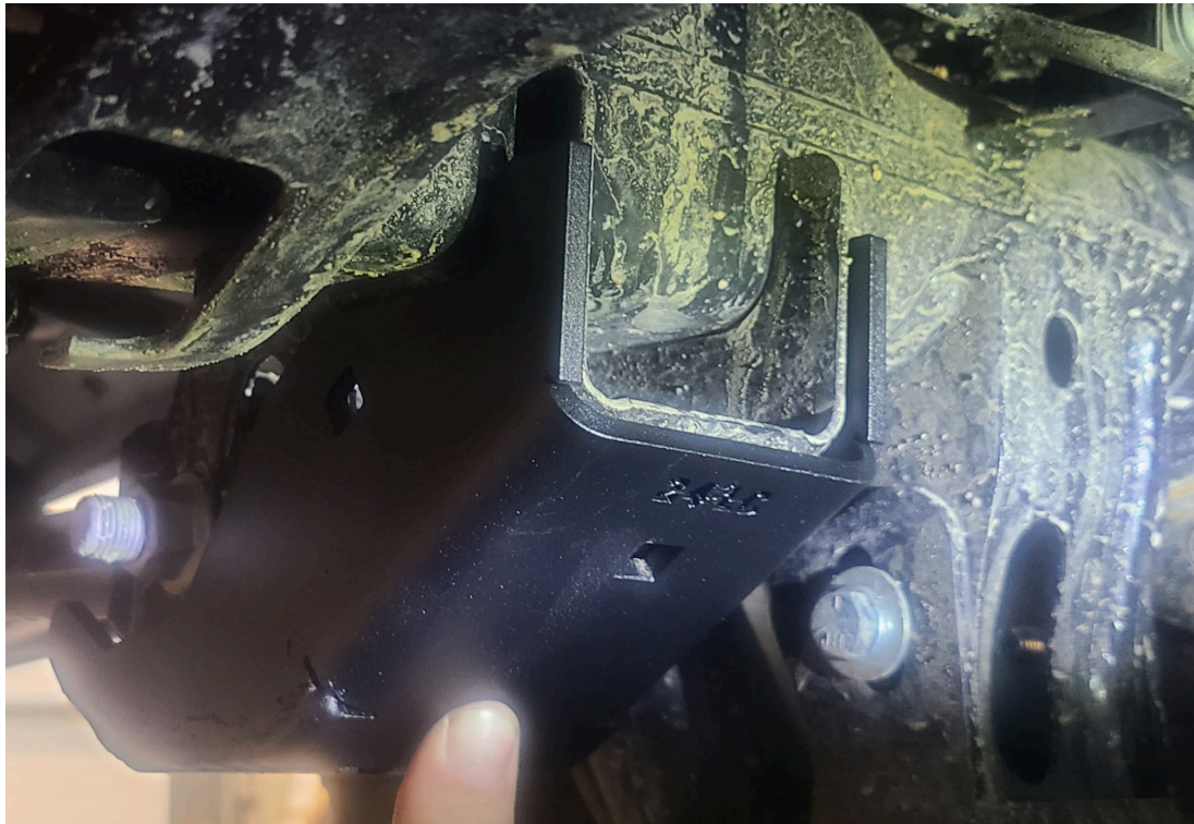
Figure 1: Holding skid up to rear link mount.
