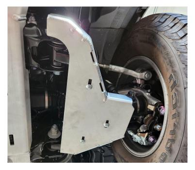
6) After the skid plate is fully installed, repeat the installation process for the opposite side.
