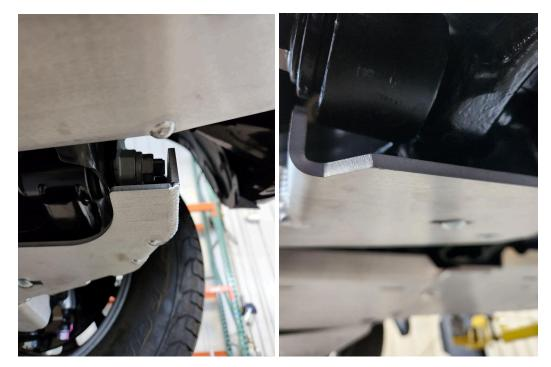
5) Once the skid is aligned properly, fully tighten all hardware.
