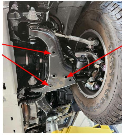
Hole for 3/8" x 4.5" Carriage Bolt
