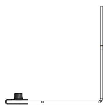
6) At the second dimple in the mounting plate bend it at a 90° angle to the left of the mounting hole as depicted below.
