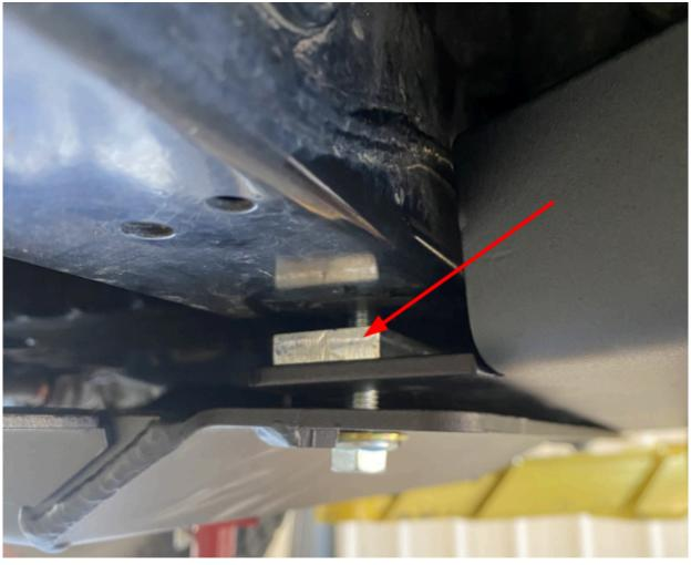
13) Align the skid plate and fully tighten all mounting bolts.
