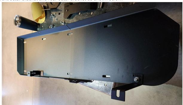
a. The front outer bracket should be installed with the outer edge of the bracket parallel with the outer edge of the skid plate.
