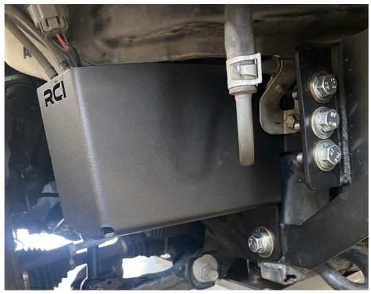
6. Congratulations! You have successfully completed installation of the RCI 10+ 4Runner Washer Fluid Reservoir Skid Plate. Take a moment to admire your work and ensure all hardware is tightened.
