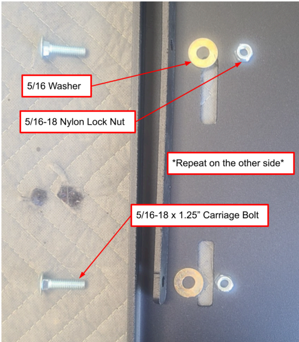
Figure 9: Engine Brace Assembly.
