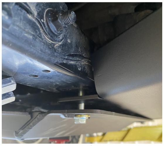
11) Use the M10 and M8 bolts to secure the back of the skid plate to the truck.
