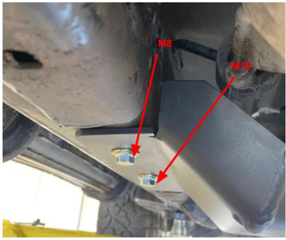
12) With the skid plate loseley installed, collect the two (2) 3/8 " transmission spacers and install them between the skid plate and the crossmember as shown below.
