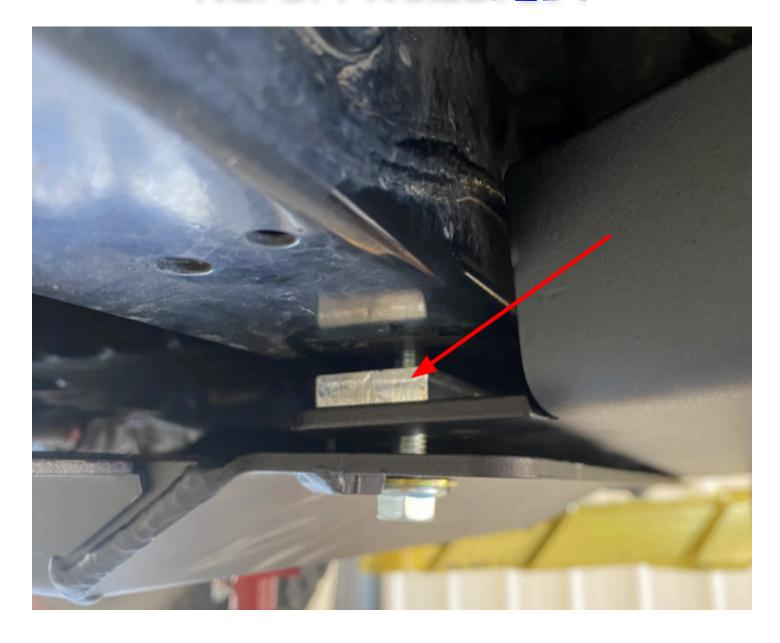
13) Align the skid plate and fully tighten all 4 mounting bolts.
