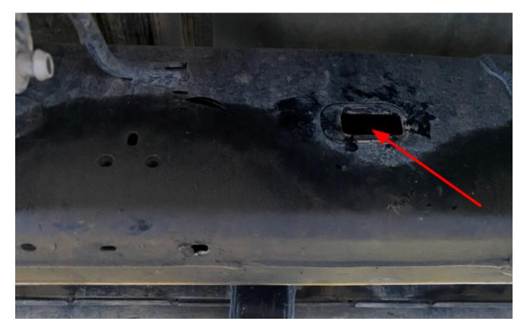
8) Insert the assembled MP4 into the slot in the frame and align the threads with the hole on the bottom of the frame.
