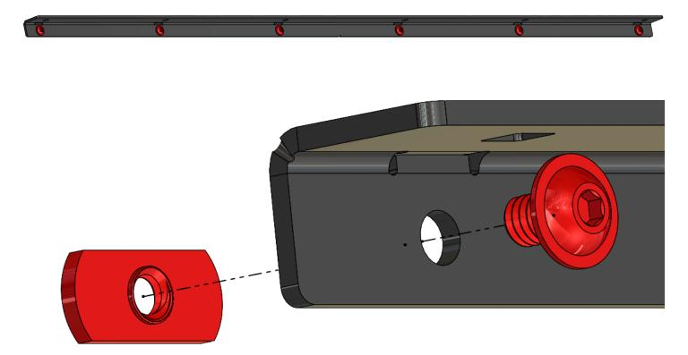
5. From the side, slide the t-slot nuts into the slots of the extrusion crossbar.
