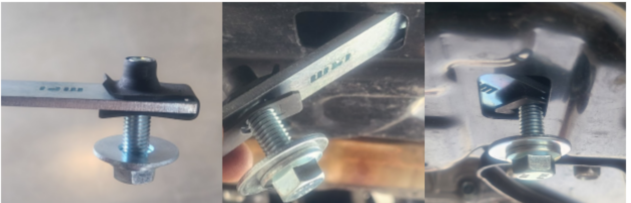
1: Partially thread bolt.
