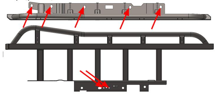
8. With the holes aligned, reinstall the fuel tank front bracket with the OEM M8 hardware. Then, remove an M8 bolt from the tapped plate within the frame, taking care not to disturb the plate(Marked with blue arrows). Reinstall the M8 bolt with a 5/16" flat washer and 5/16" fender washer. Repeat the process with the remaining M8 bolt.
