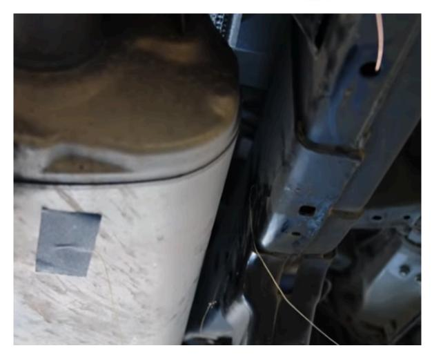
e. Insert the tapped plate, use the strings to align the thread holes with the third and fourth holes in the underside of the driver frame, and loosely thread another pair of M8 bolts into the plate.
