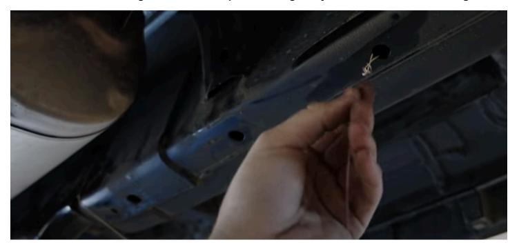
d. Repeat the process of passing the wire through the 4th hole on the underside of the frame, tie the string to the loop on the end of the wire, and pull the string through.
