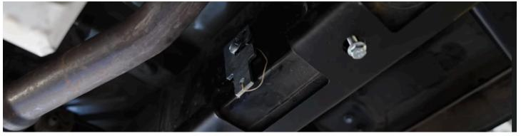
b. The first 7/16" carriage bolt is placed within the rectangular slot behind the crossmember.
