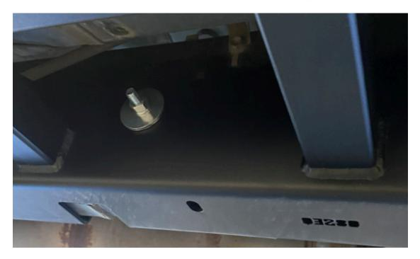
Apply upward pressure on the slider frame plate so that it is resting on the bottom of the frame. Fully tighten the three 7/16" carriage bolts.
