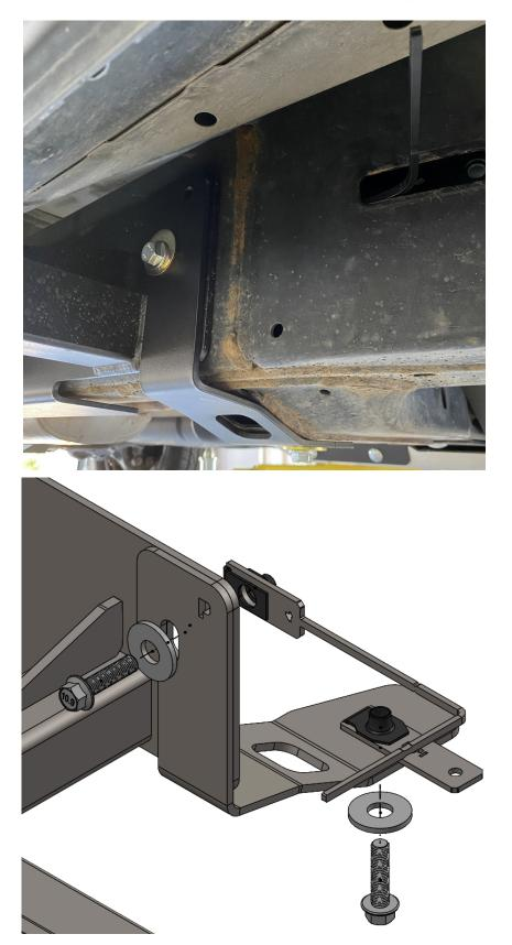
17) Apply upward pressure and fully tighten both M10 bolts.
