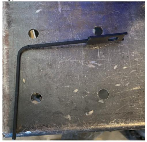
9) Install one M10 speed clip on the mounting plate.
