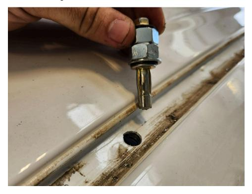
26. Apply a generous amount of sealant to the mounting flange and slotted area of the stem of a plus nut.
