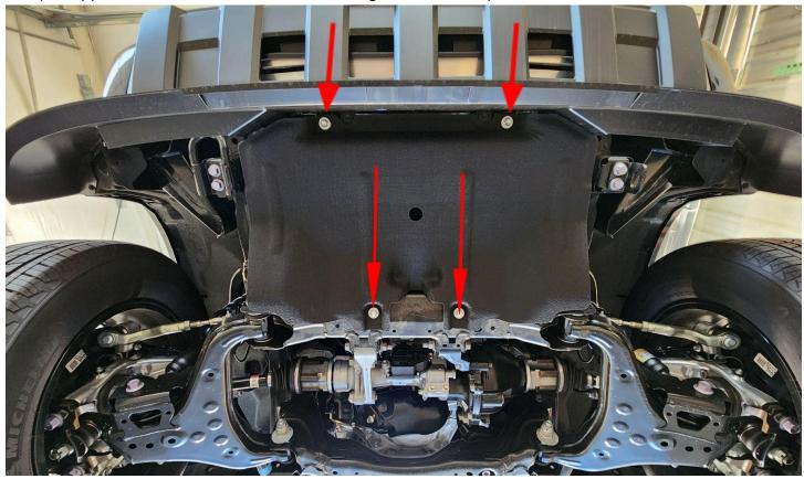
4) Remove the 4 purple M12 bolts securing the factory recovery points to the lower horns on the vehicle frame.
