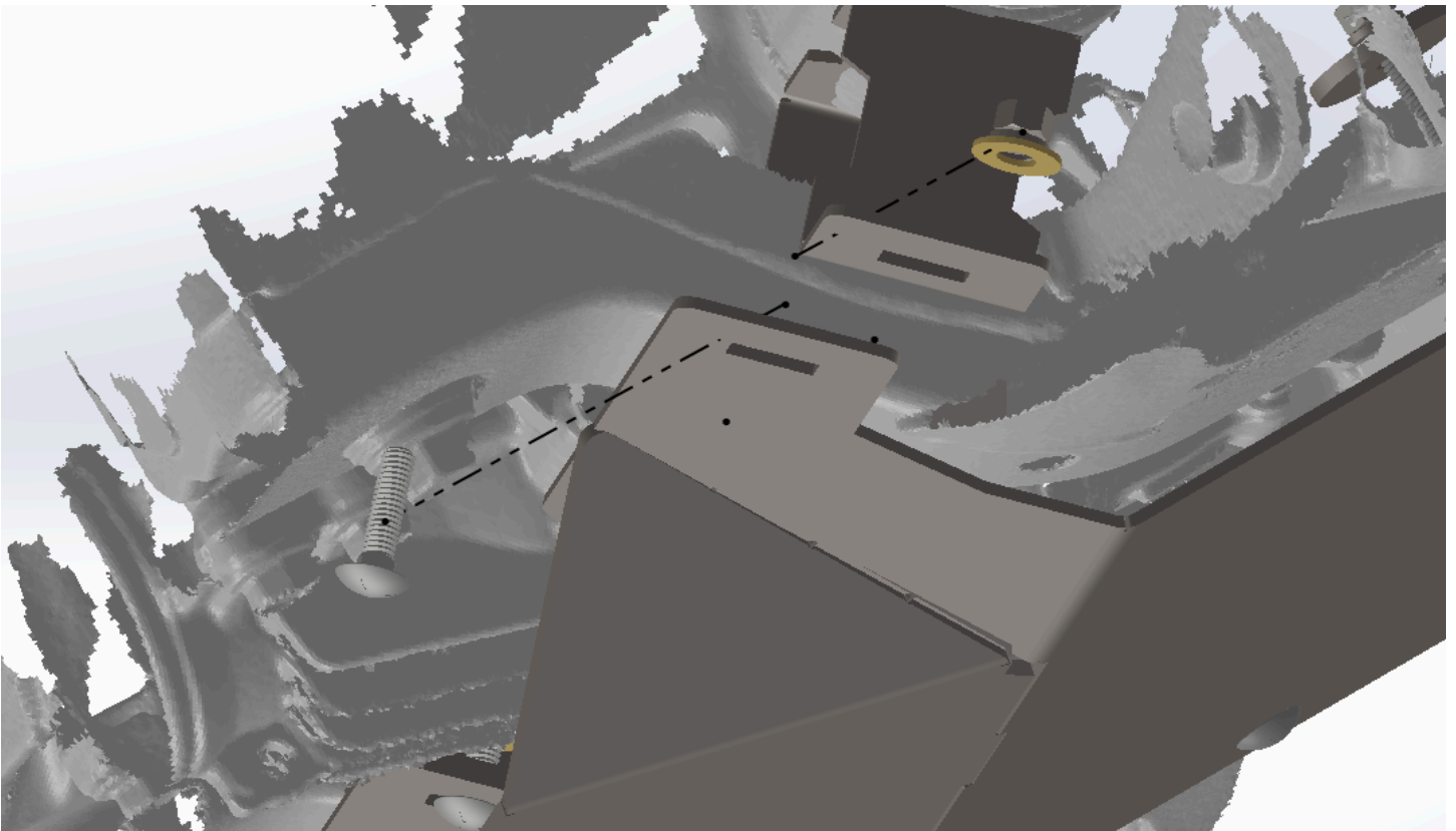
Figure 4: Diff Clamp Assembly.
