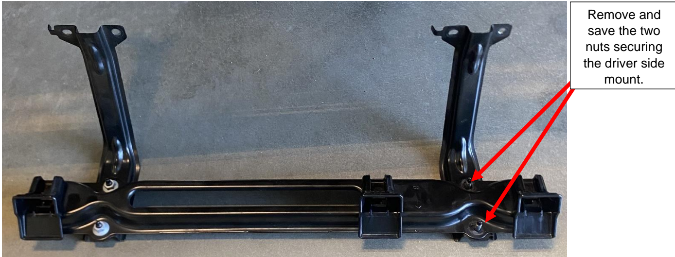
Figure 25: Remove the driver side mount.
