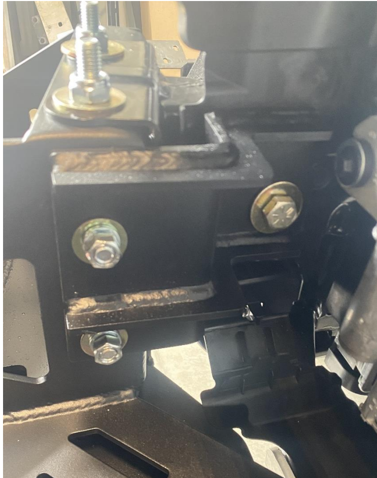
Figure 23: Correct installation of secondary bracket.
