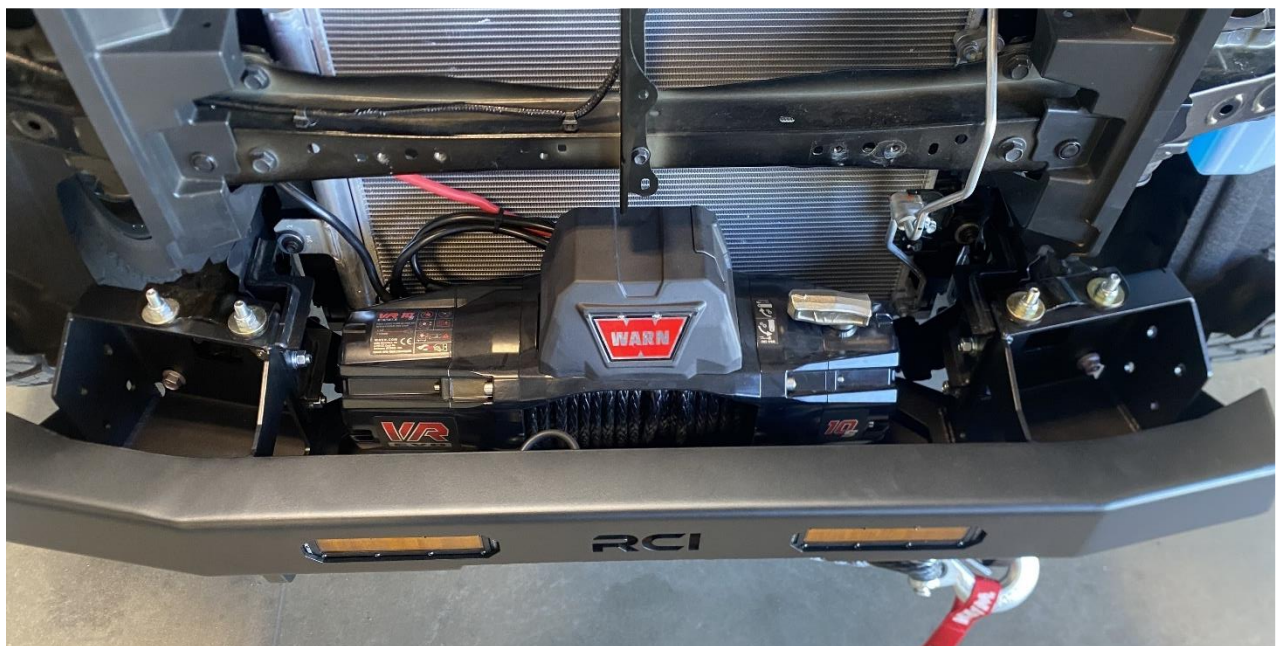
Figure 24: Example of winch and lights installed.
