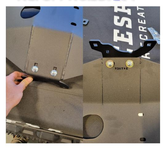
3. Using another set of the included 3/8" x 1" carriage bolt, washer, split washer, and nut, loosely secure the upper pinion clamp to the lower pinion clamp.
