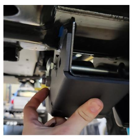
4. Loosely thread the included flat washer, split washer, and nut onto the carriage bolts.
