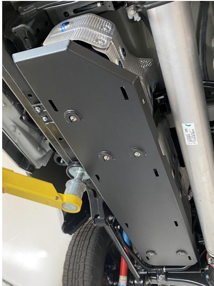
Figure 3: Correctly installed fuel tank skid plate.
