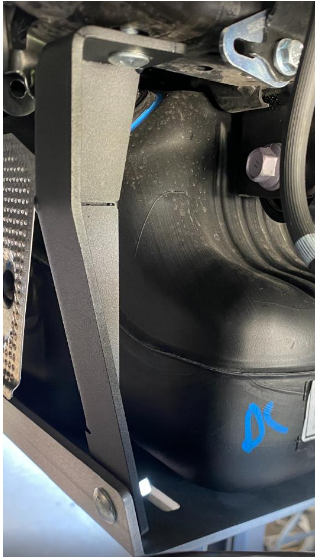
Figure 13: Correctly installed rear driver bracket.
