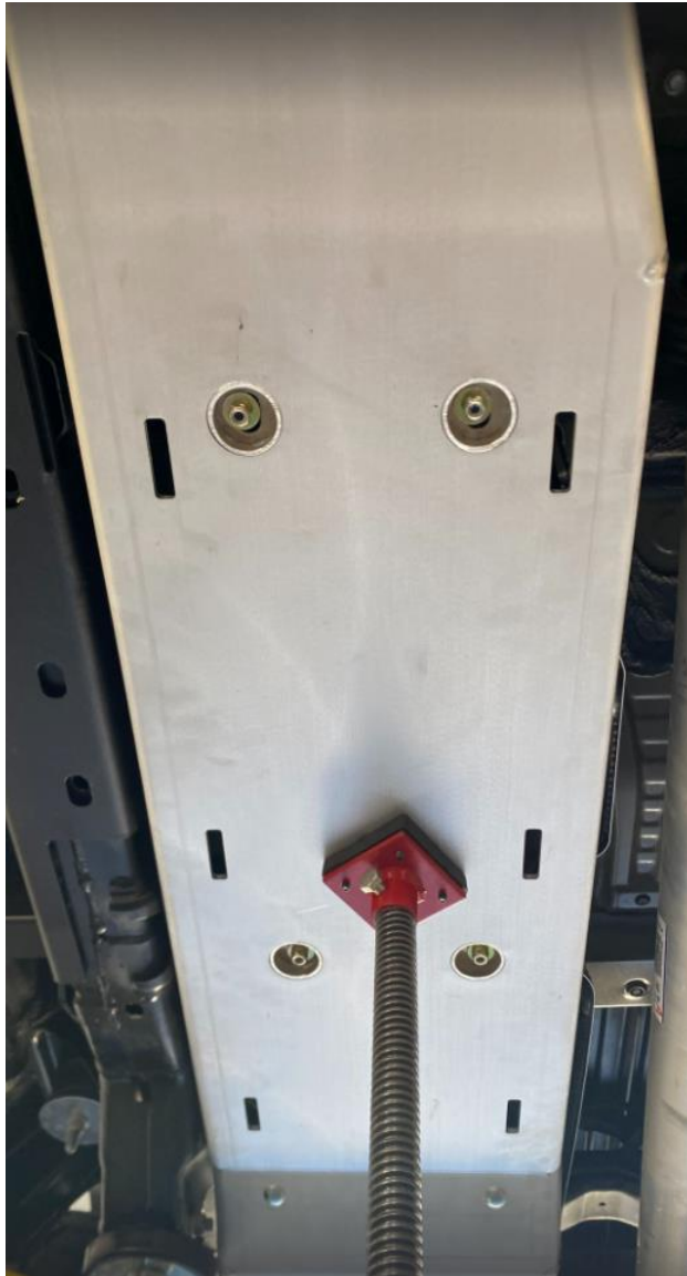
Figure 8: Skid plate loosely installed with M8 nuts.
