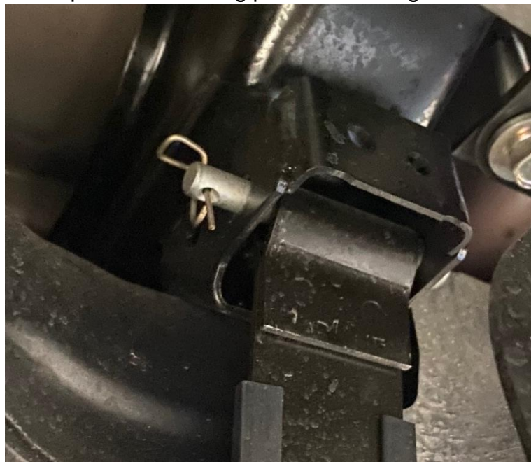
Figure 15: Driver Side Pin and Retaining Pin
