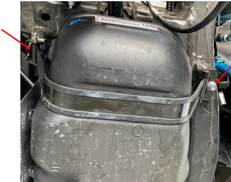
Figure 4: Remove rear fuel tank strap.
