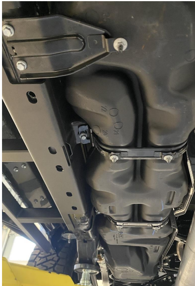
Figure 2: Fuel tank with skid removed.
