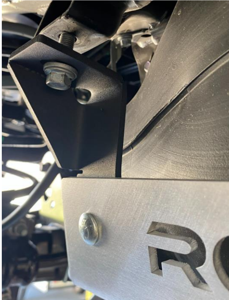
Figure 11: Correct installation of rear passenger bracket.
