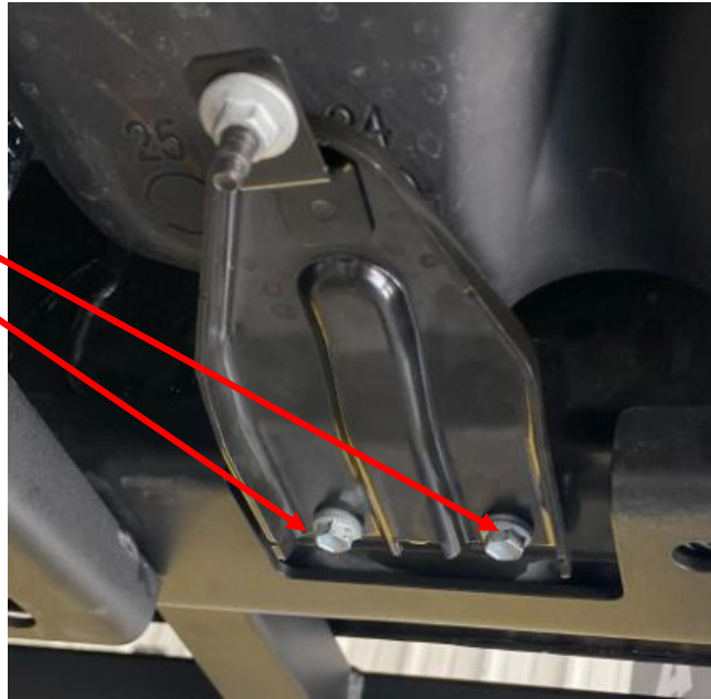
Figure 3: Remove front mounting bracket.
