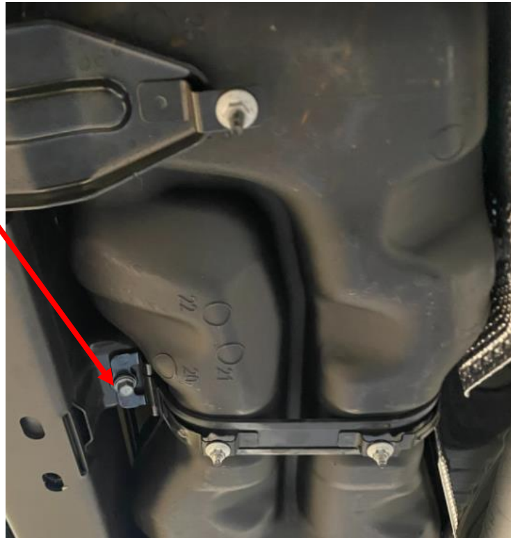
Figure 14: Mounting bolt to remove.
