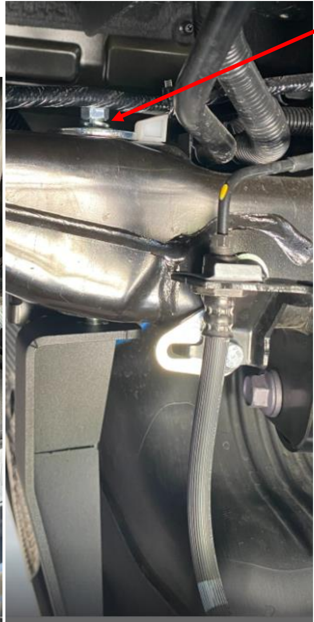
Figure 13: Correctly installed rear driver bracket.
