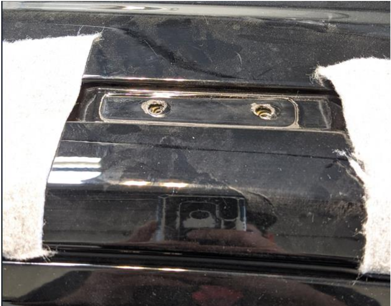
Figure 3: Roof Mounting Holes With tape cut
