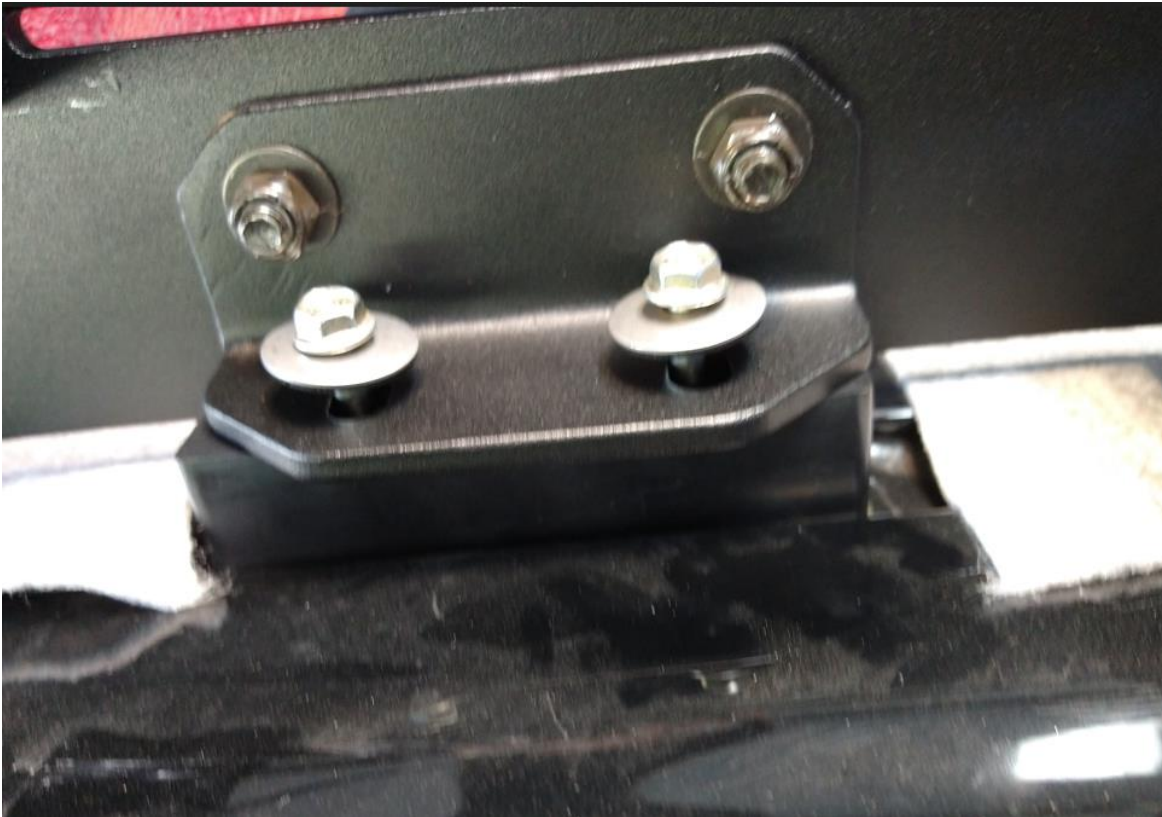
Figure 16: Correct Roof Rack/Rubber Block Install.
