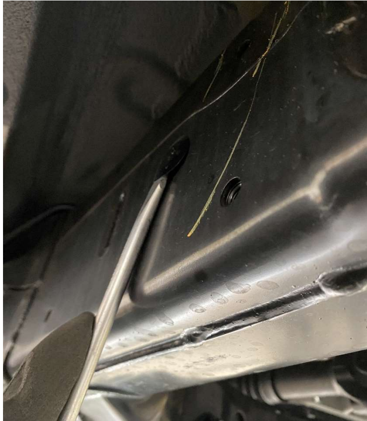
Figure 3: Pry off the plastic clips.
