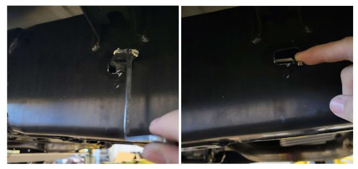
Align the M10 speed clips with the holes in the bottom face of the vehicle frame.
