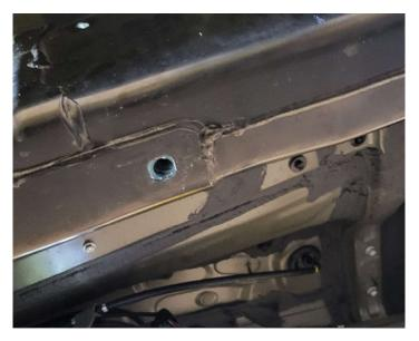
e. Align the transfer case crossmember with the holes in the bottom face of the vehicle frame and support the center with a floor jack or similar.
