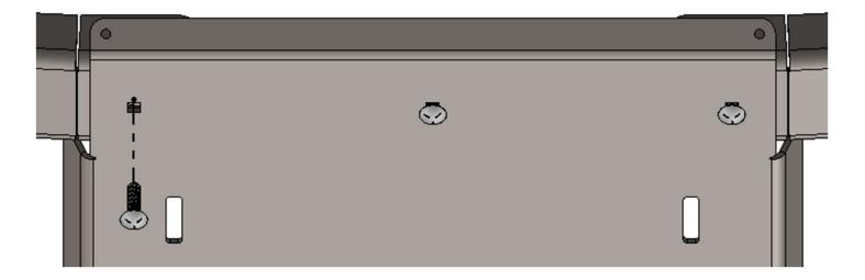
7) Slide the included 3/8" transmission spacers between the vehicle crossmember and the front mounting face of the RCI 24+ Tacoma Transfer Case Skid Plate and tighten all hardware.
