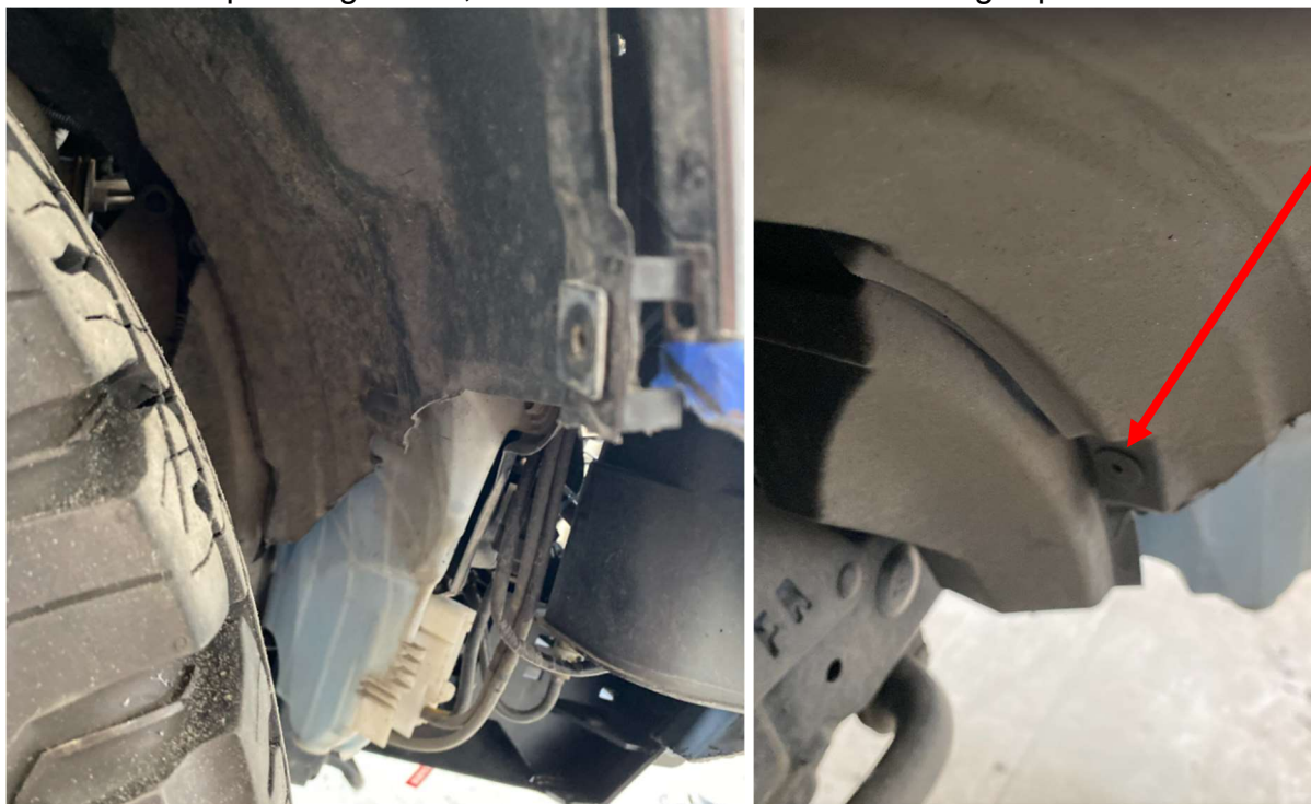
Figure 11: Passenger side wheel well trim example.
