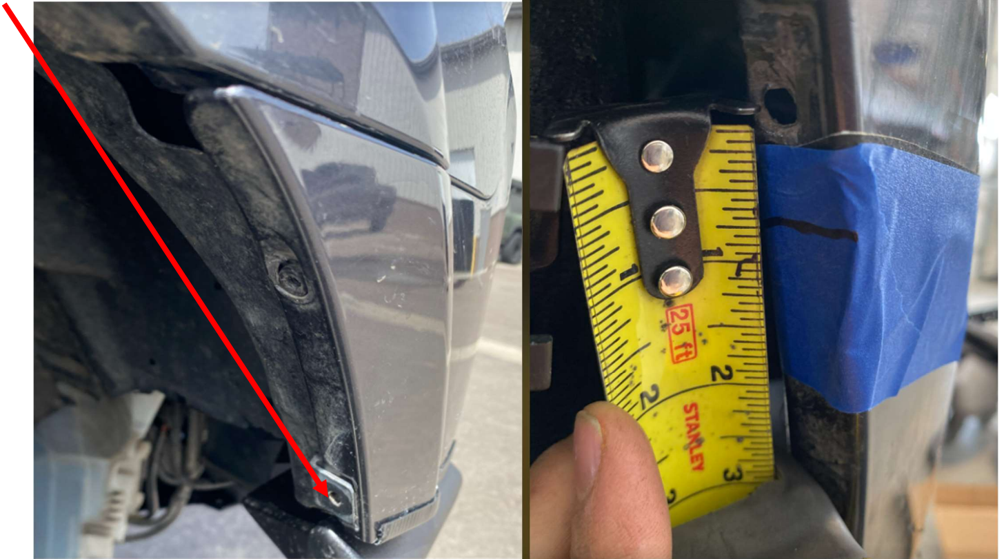
Figure 7: Mark a line \frac{3}{4} " down from second highest fender liner hole.
