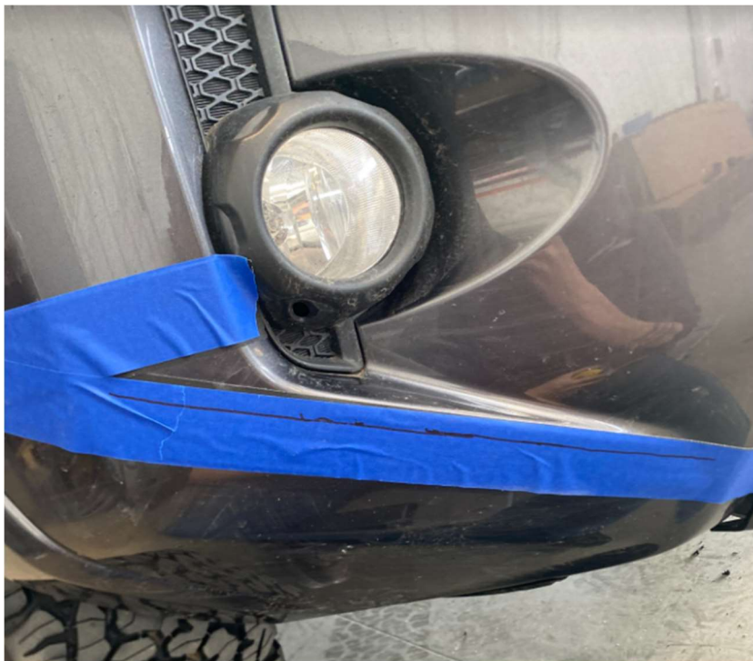
Figure 6: Template correctly installed on bumper.
