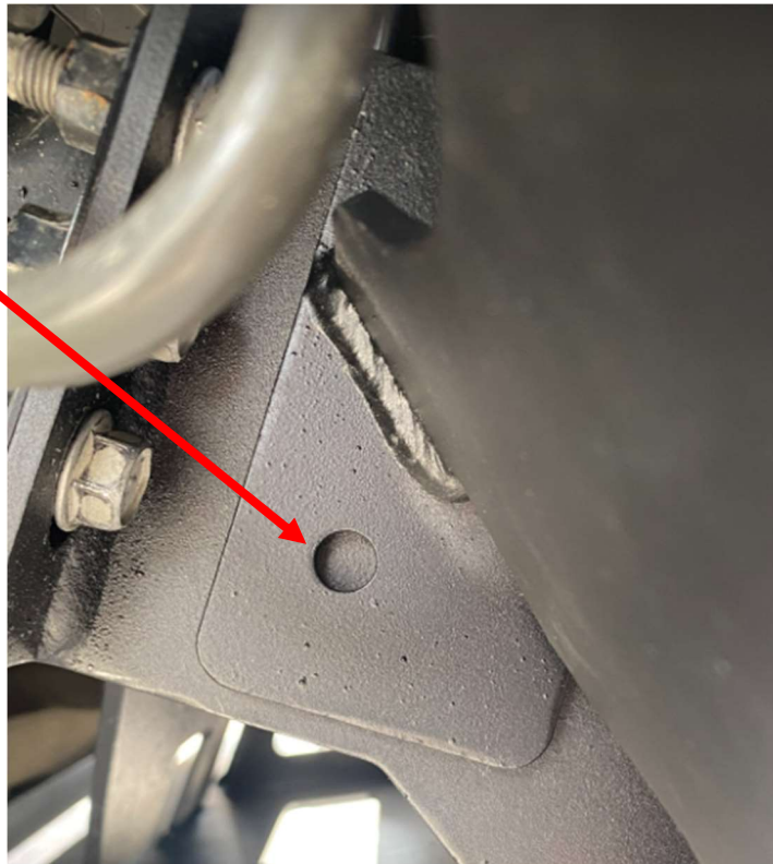
Figure 17: If old style bumper, drill out a 3/8" hole.
