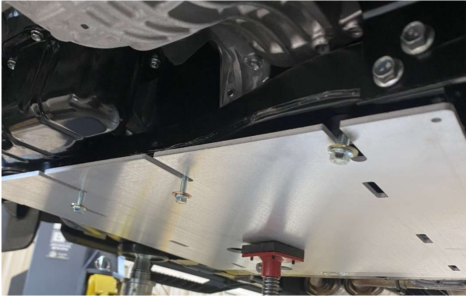
Figure 3: Front mounting of transmission skid.
