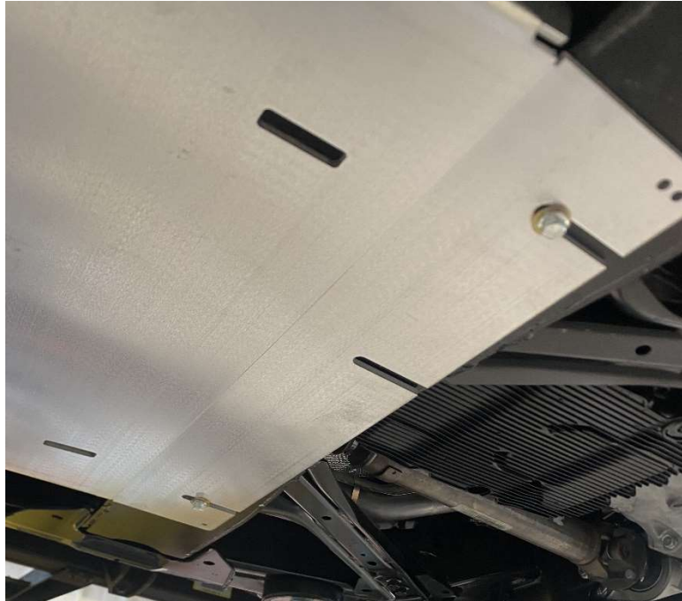
Figure 5: Front mounting of t-case skid.
