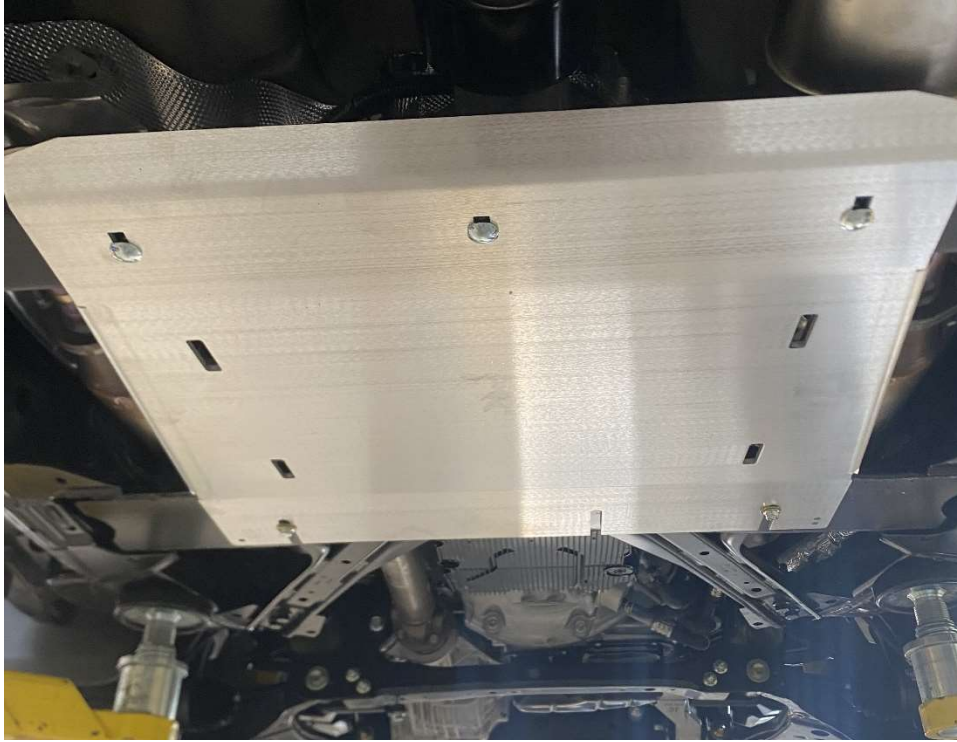
Figure 6: Correctly installed t-case skid.
