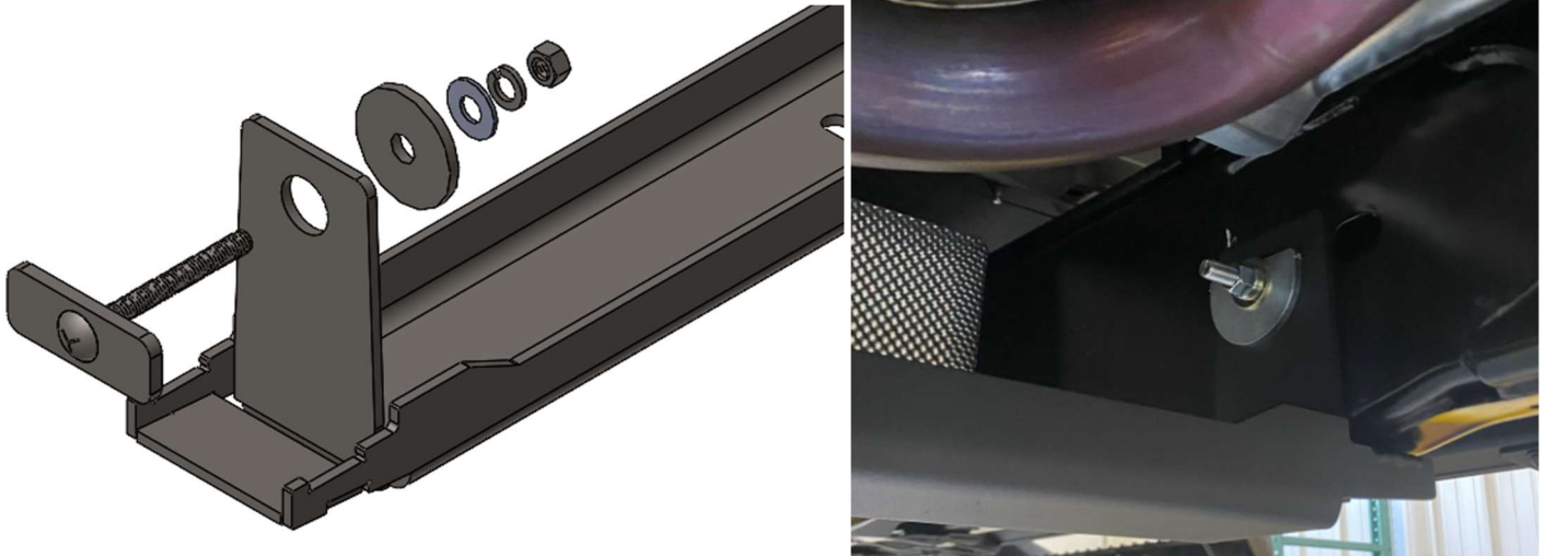
Figure 2: Crossmember hardware orientation.
