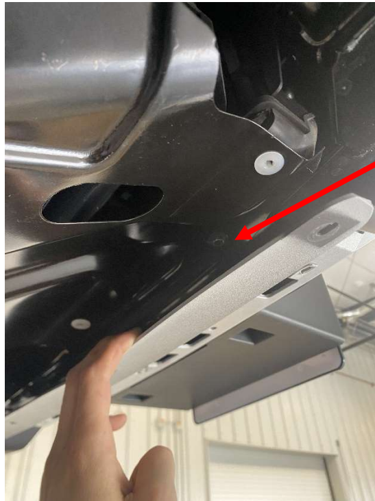
Figure 6: Engine skid bolt location.
