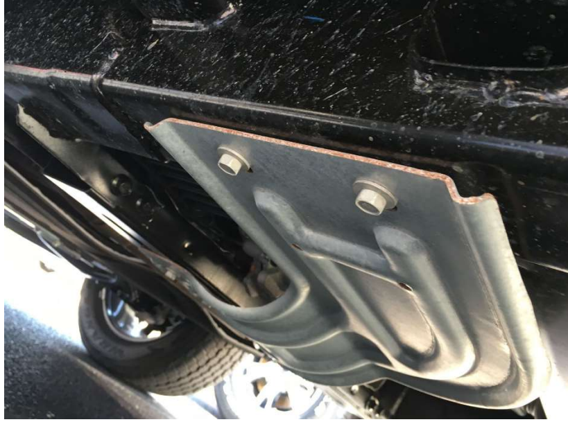
Figure 2: OEM Transfer Case Skid to be Removed.
