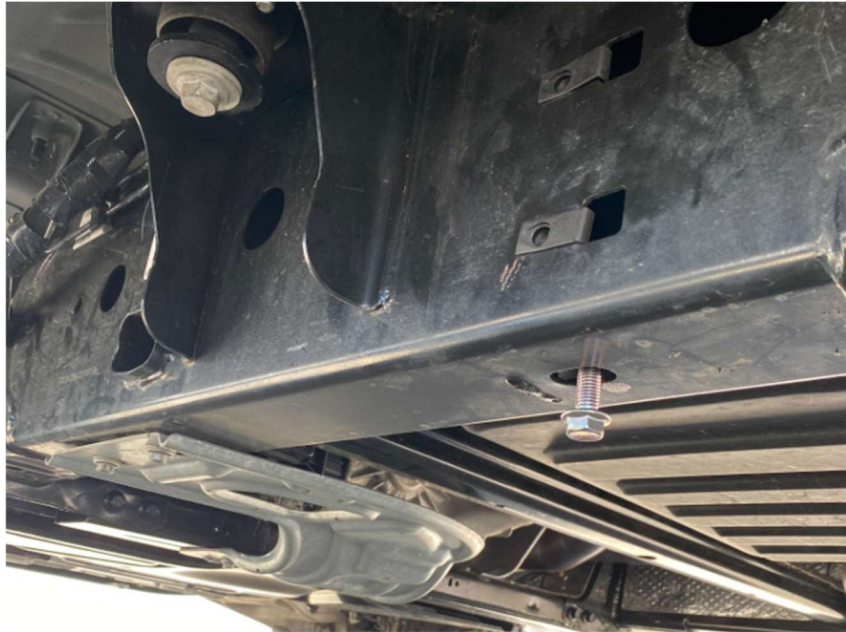
Figure 7: Preinstallation of Lower M10 Bolt
