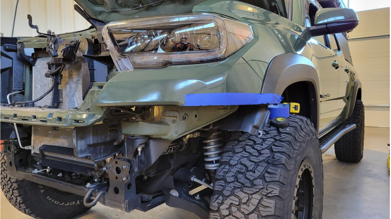
Figure 6: Completed cut on driver side
