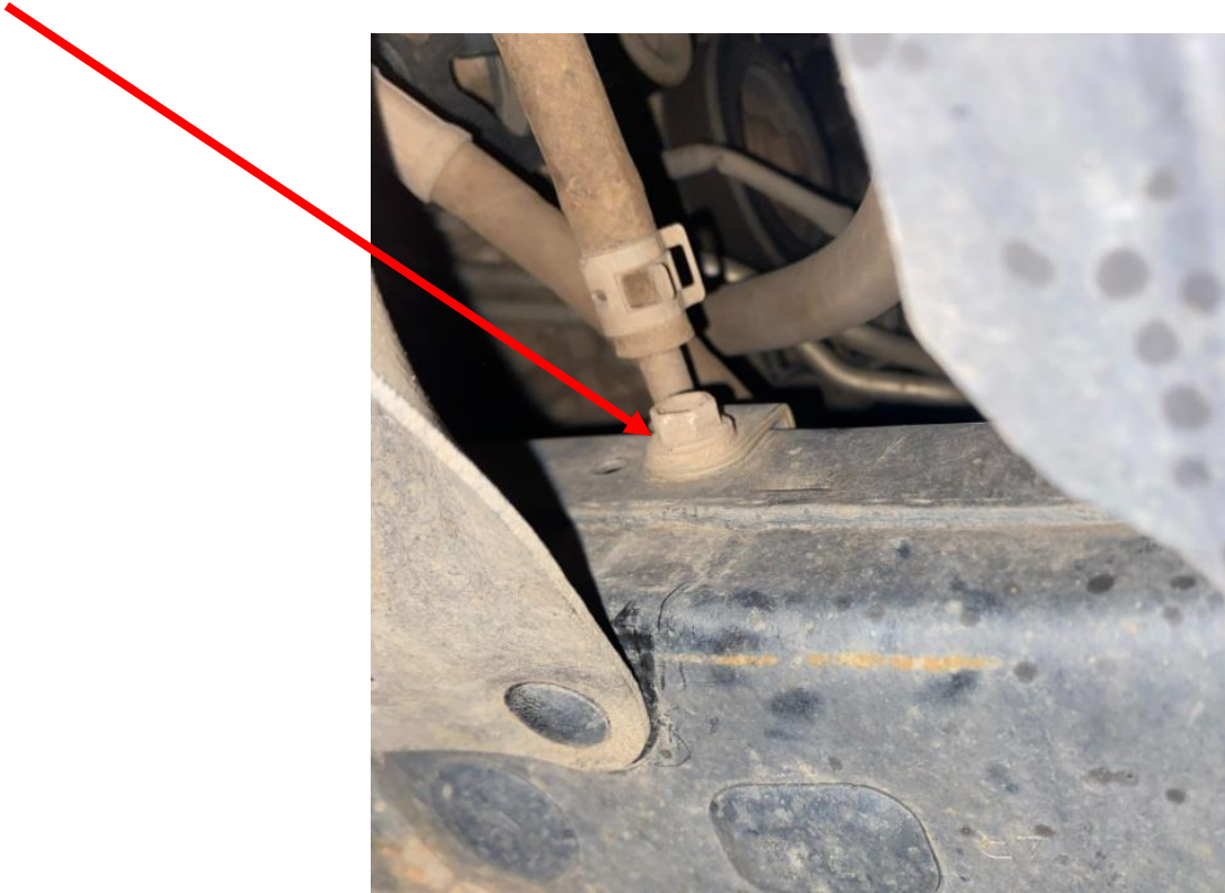
Figure 10: Mount located behind passenger wheel well splash guard.
