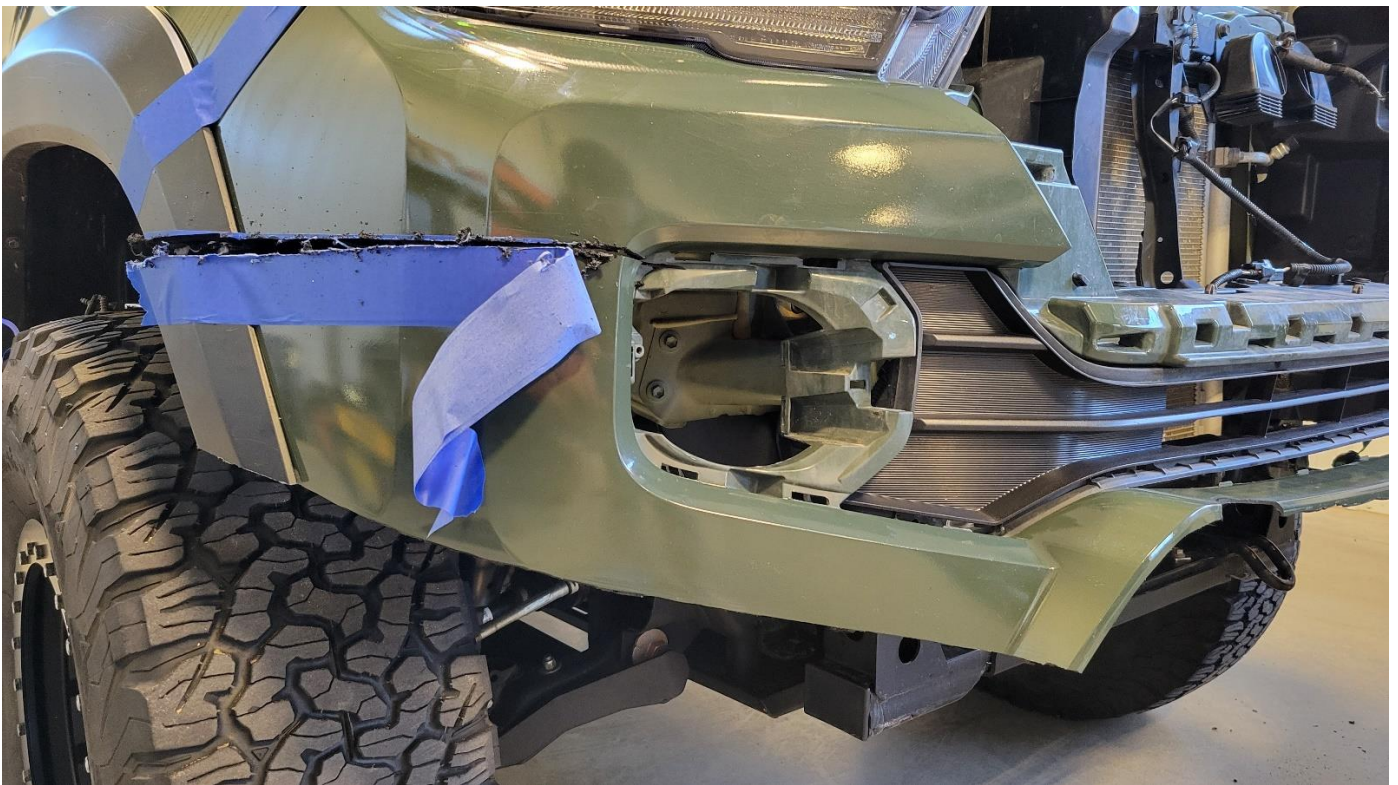
Figure 5: Partially completed passenger side cut
