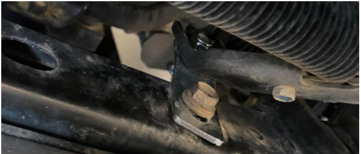
Figure 13: Correct installation of frontmost brackets.
