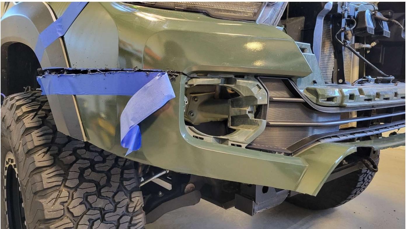
Figure 5: Partially completed passenger side cut
