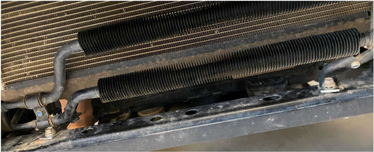
Figure 14: Correct installation of frontmost brackets.
