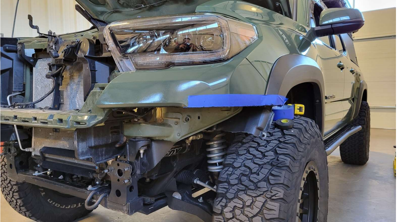
Figure 6: Completed cut on driver side
