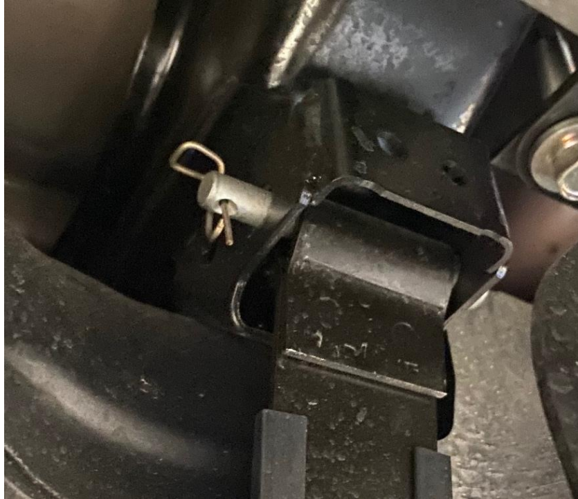
Figure 9 Driver Side Pin and Retaining Pin
