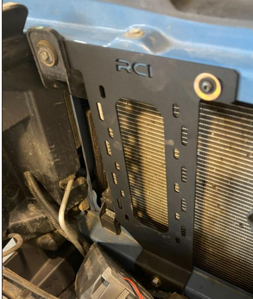
Figure 4: Correct Installation of Relocation Bracket.
