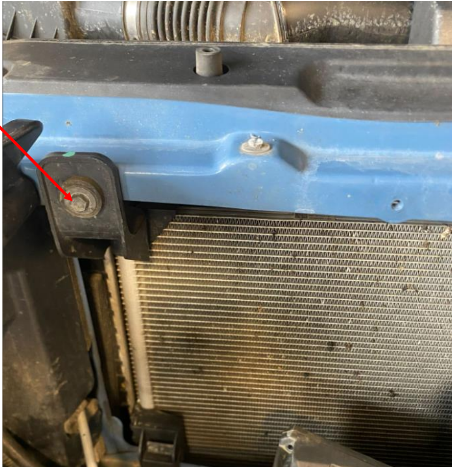
Figure 3: Fastener to be Removed.
