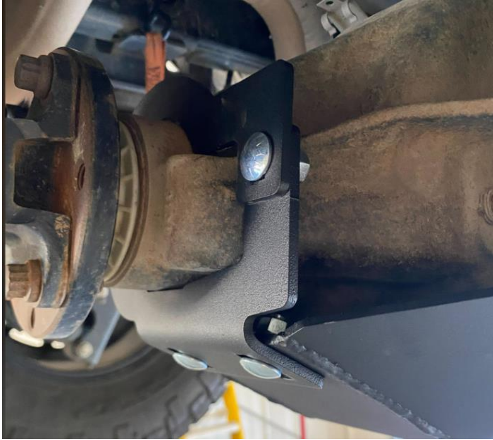
Figure 6: Pinion Clamp Installation
