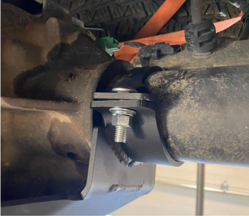
Figure 8: Axle Clamp Installation
