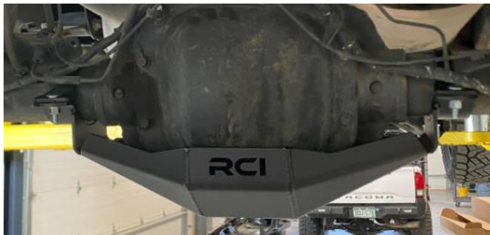
Figure 8: Correct Installation of Diff Skid
