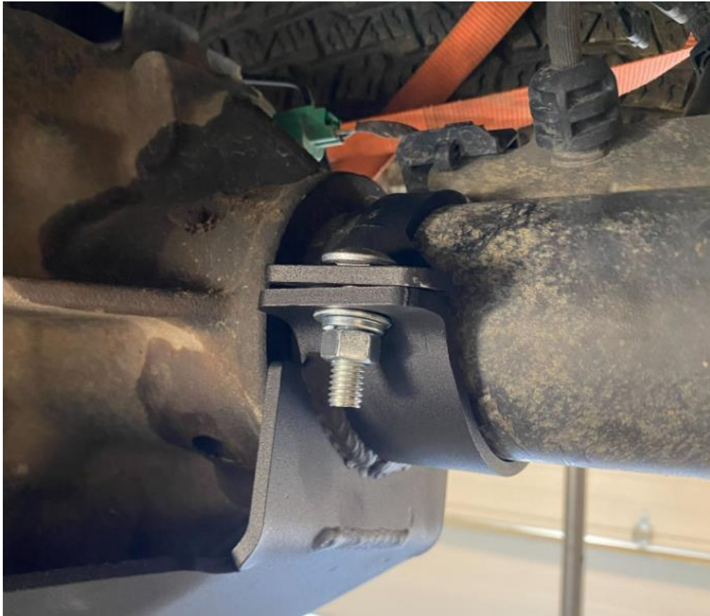
Figure 7: Axle Clamp Installation
