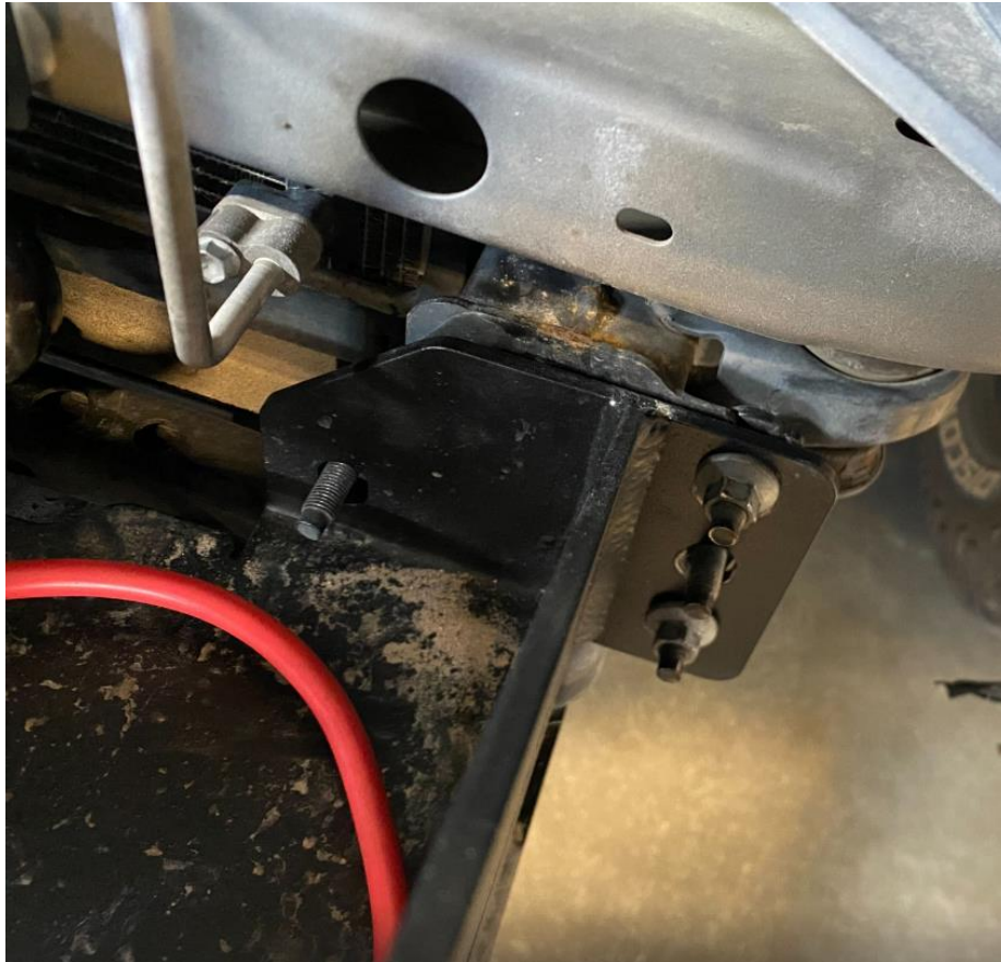
Figure 9: Correct installation of bumper on mounting surface
