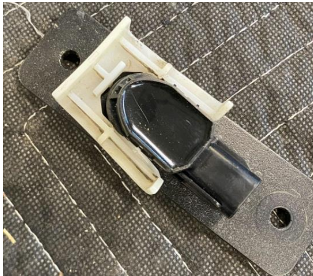
Figure 4: Example of parking sensor installed (Ignore bracket in model, parking sensor will be mounted directly to the bumper)
