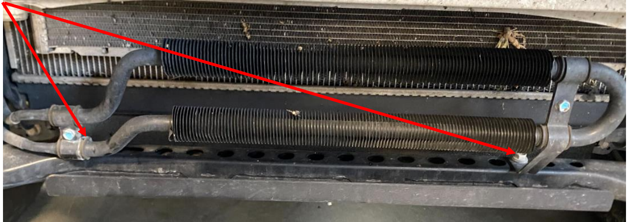
Figure 5: Remove the two M8 bolts securing the radiator
