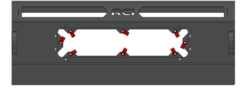
b. Use 8 of the included m8 button head bolts to secure the center filler panel to the center section of the RCI Bronco bumper.
